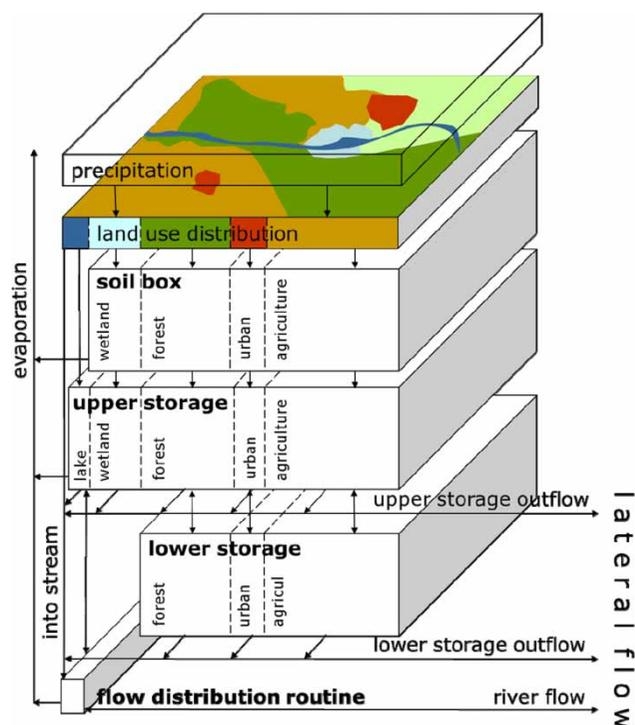
**Figure 2** | Schematic representation of the sub-grid parameterization scheme in a single model grid cell. All water flows and storages within the model routines are weighted according to their designated land use class. Vertical flows indicate fluxes between different model storage compartments. Lateral flows indicate fluxes to neighbouring draining grid cells.
