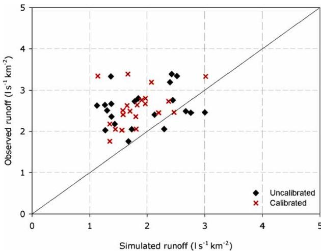
**Figure 7** | Validation of the model performance by comparison of synoptic specific discharge measurements with simulated synoptic specific discharge (uncalibrated:  $r = 0.22$ ; calibrated on synoptic measurements:  $r = 0.36$ ).
