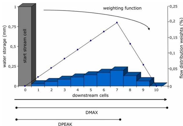
**Figure 3** | Downstream distribution of stream water according to the flow distribution parameters DMAX and DPEAK of the flow routing routine.
