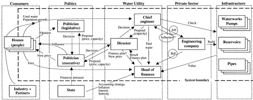
Figure 2 Model diagram showing the water supply system of a city in Switzerland in a simplified and abstract form. The model is constructed with an agent-based, hierarchical and variable structure
