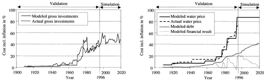
Figure 4 Validation of modeled financial parameters such as investments (left) and water price (right). Simulation up to 2020 assuming the same rules and capacity development as in Figure 3. Modeled debt and financial result are shown (right) for later comparison with Figure 5
