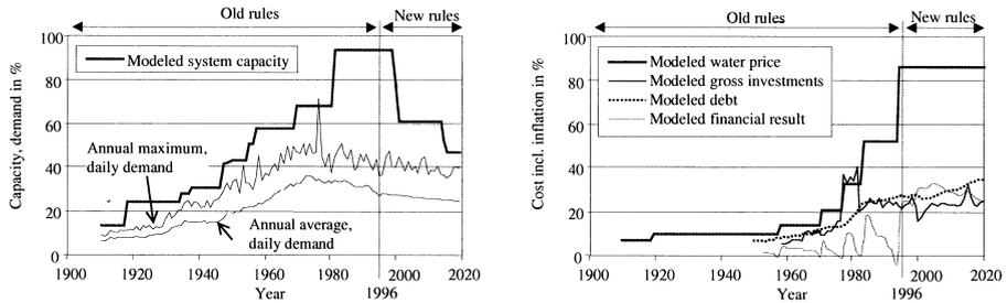
Figure 5 Simulation of a scenario in which the rules of the utility engineer and the engineering company (see Figure 2) are changed. Left – effect of new rules on capacity, right – on financial parameters. This scenario can be compared to the ones in Figures 3 and 4
