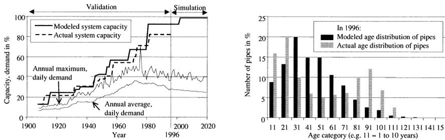
Figure 3 Left: validation of modeled system capacity up to 1996, and simulation up to 2020 assuming the same rules as in the past and a decreasing average demand trend respectively. Right: validation of age distribution of the pipes for the year 1996
