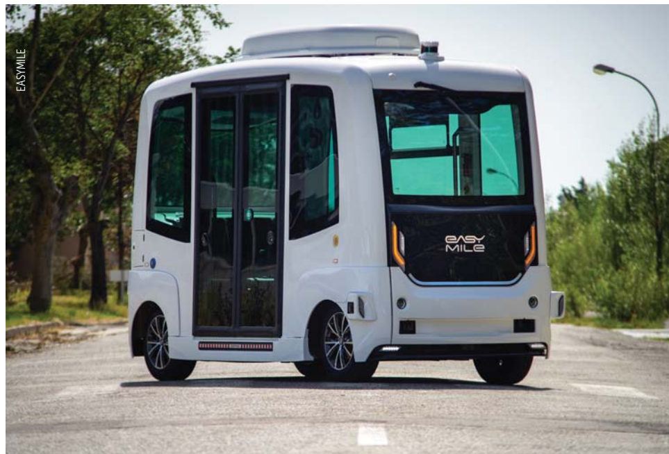
A SELF-DRIVING SHUTTLE identical to the one shown here by EasyMile, a company headquartered in Toulouse, France, was tested earlier this year by the Regional Transportation District in Denver, Colorado. Snow and heavy rain confused the onboard sensors, disrupting the shuttle service.
