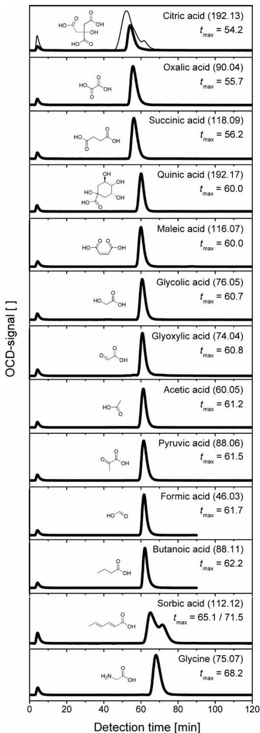
**Figure 2** | SEC-OCD bypass peaks, chromatograms and chemical structures of various low molecular weight aliphatic and cyclic mono-, di- and tricarboxylic acids without and with further functional groups and molecular weights in brackets and  $t_{\max}$  in min (humic acid indicated as weak line in the chromatogram of citric acid). Acids are indicated since names of their carboxylates are used less.
