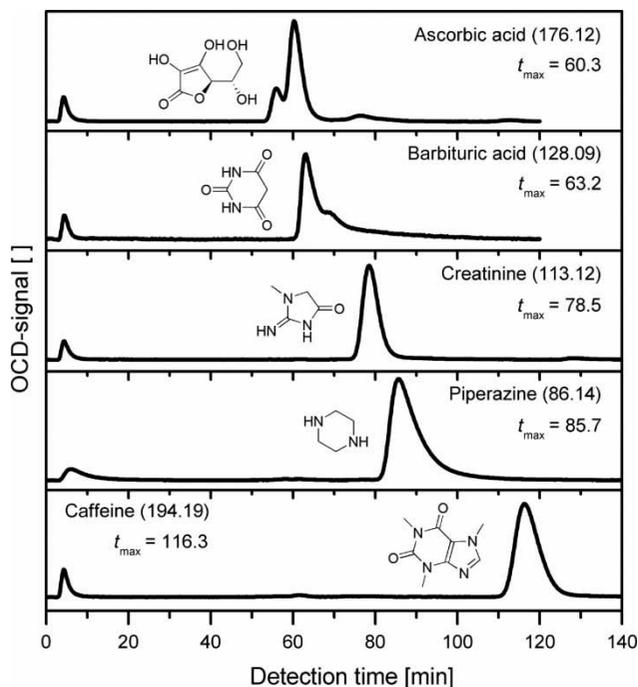
**Figure 4** | SEC-OCD bypass peaks, chromatograms and chemical structures of heterocyclic (non-carboxylic) organic compounds (molecular weights in brackets).
