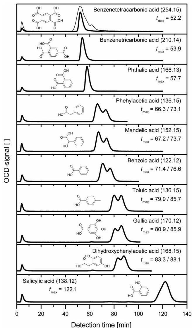
**Figure 3** | SEC-OCD bypass peaks and chromatograms and chemical structures of different low molecular weight aromatic carboxylates (molecular weight of acids in brackets and indicated peak detection time  $t_{max}$  in min) with up to four carboxylic functional groups (humic acid included as weak line in the chromatogram of benzenetetracarboxic acid). Names of acids instead of carboxylates are indicated for simplification.
