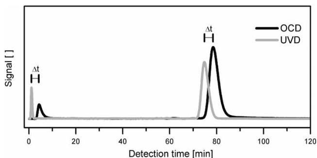
**Figure 6** | SEC-OCD and SEC-OCD bypass and chromatograms of a UV active compound with indicated time lag ( $\Delta t$ ) between UVD and OCD maximum response for creatinine.
