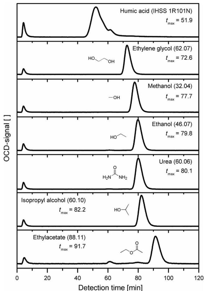
**Figure 1** | SEC-OCD bypass peaks and chromatograms of a large molecular weight model substance (Suwannee River aquatic NOM 1R101N) and hydrophilic non-carboxylate low molecular weight compounds with different functional groups (molecular weight in brackets and detection time of peak maxima  $t_{\max}$ ).
