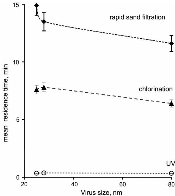
**Figure 3** | Mean virus residence time as a function of its size in rapid sand filtration, chlorination and UV treatments.
