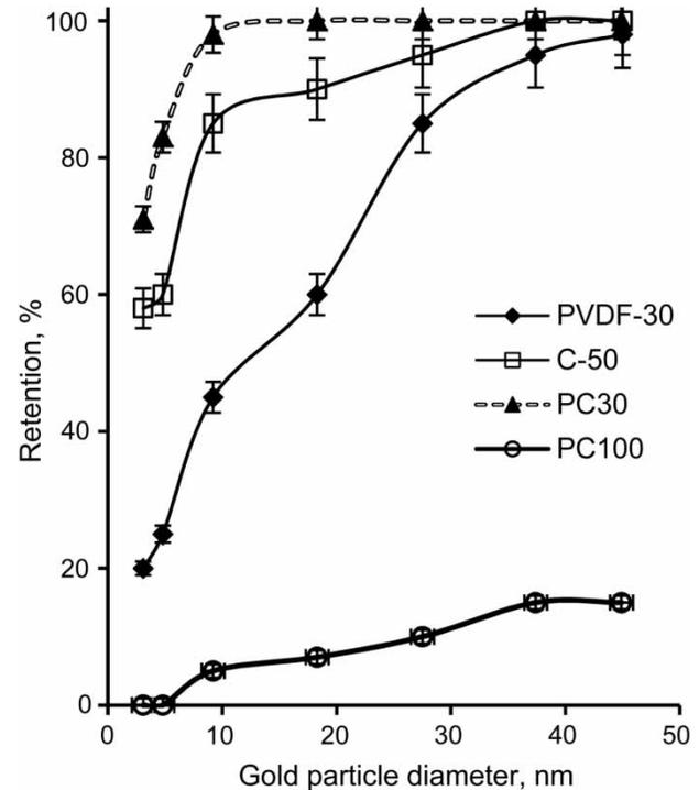
**Figure 2** | Percentage of gold nanoparticle rejection by PVDF-30, C-50, PC-30 and PC-100 membranes.
