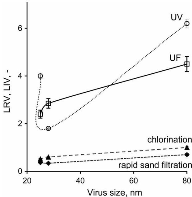
**Figure 1** | LRV and LIV values as a function of virus size. Experimental conditions: UV – 30 mJ/cm<sup>2</sup>; UF – PES-30, TMP 2 bars; rapid sand filtration – 100 cm depth; chlorination – 2 mg/L free chlorine, contact time 2 min. The UF of VV resulted in 6 LRV (not shown).
