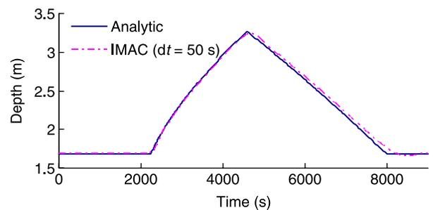
Figure 5 | Simulation hydrograph of depth for channel flow.
