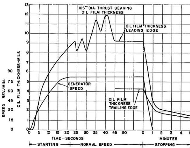
FIG. 14 TEST RESULTS ON PIVOTED-PAD THRUST BEARINGS
