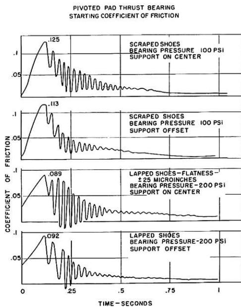
FIG. 15 STARTING COEFFICIENT OF FRICTION FOR PIVOTED-PAD THRUST BEARING
