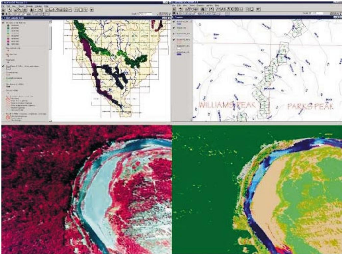
**Figure 4** | Top left: flight line tracking of aerial digital multi-spectral sensing aircraft; top right: GIS coverage of individual image ground footprints for a single flight line; bottom left: three-band false colour composite digital multi-spectral image of the Klamath River; bottom right: GIS resource classification of digital image shown in Panel C.
