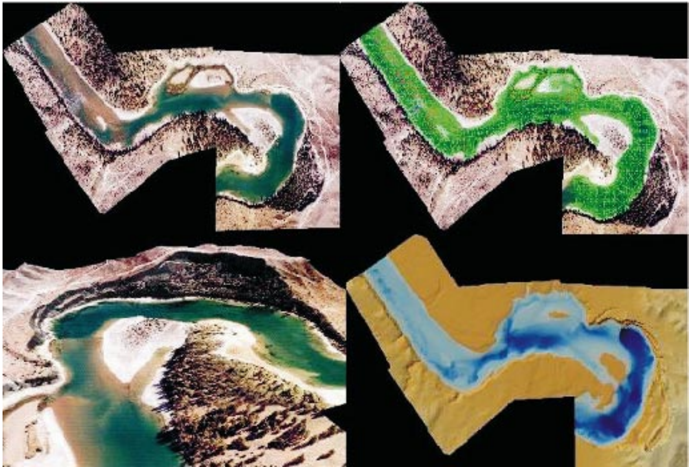
Figure 5 | Top left: high-resolution digital aerial photograph of an intensive study site used to generate digital terrain model; top right: GPS-coupled hydro-acoustic mapping tracks of channel topographies; bottom left: digital aerial photograph draped over 3-dimensional terrain model of study site; bottom right: 3-dimensional terrain relief for study reach in GIS format.
