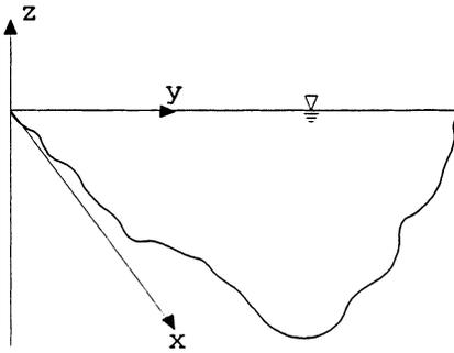
Fig. 1. A cross-section of a lake with an arbitrary bottom topography perpendicular to the shore ( $y$ -axis), but with constant depths along the shore ( $x$ -axis). The velocity and temperature fields are also considered as homogeneous along the  $x$ -axis.
