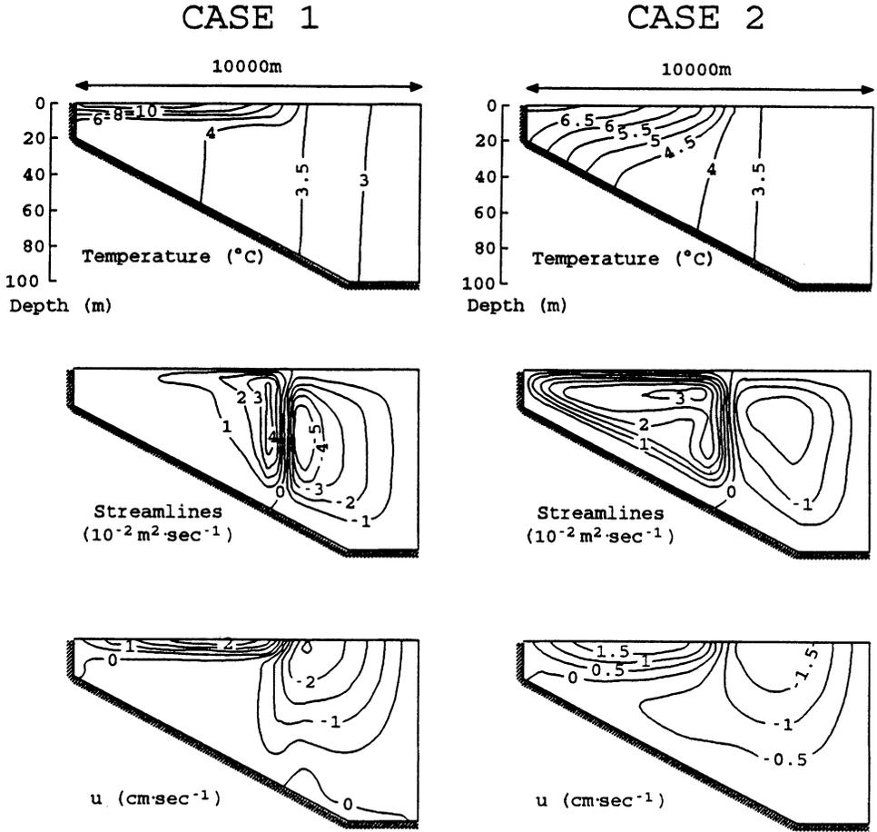
Fig. 2. Obtained temperature distributions, streamfunctions, and long-shore velocity distributions for cases 1 and 2 (section A, with the bottom slope  $10^{-2}$ ) when only density-driven currents were considered. Only half of the cross-section is shown as the center is a symmetry line.
