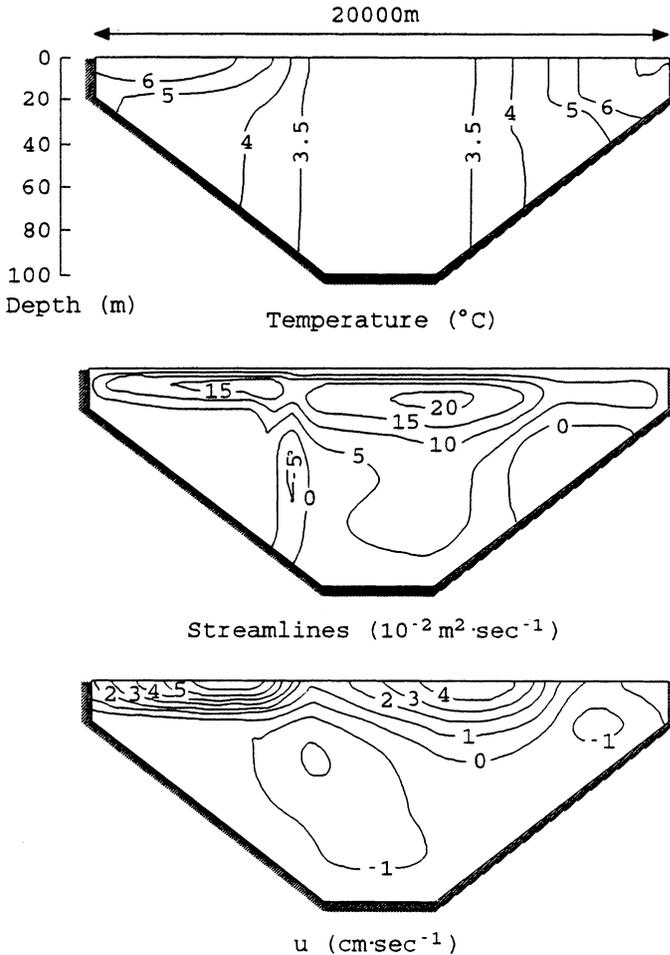
Fig. 9. Temperature distribution, streamfunction, and long-shore velocity distribution for wind- and density-driven currents for section A. The imposed wind speed is  $6 \text{ m sec}^{-1}$  along the section (from left to right).
