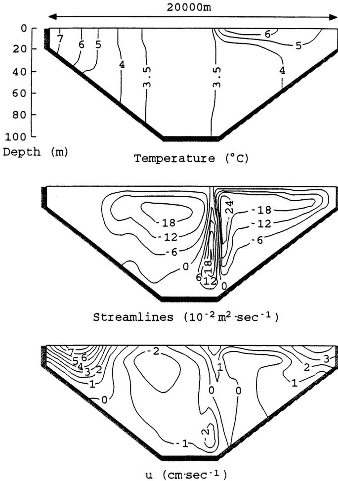
Fig. 10. Temperature distribution, streamfunction, and long-shore velocity distribution for wind- and density-driven currents for section A. The imposed wind speed is  $4 \text{ m sec}^{-1}$  along the shore line (out from the paper).
