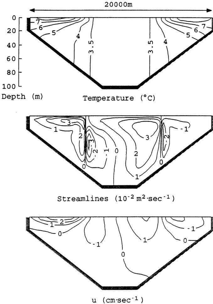
Fig. 8. Temperature distribution, streamfunction, and long-shore velocity distribution for wind- and density-driven currents for section A. The imposed wind speed is  $2 \text{ m sec}^{-1}$  along the section (from left to right).
