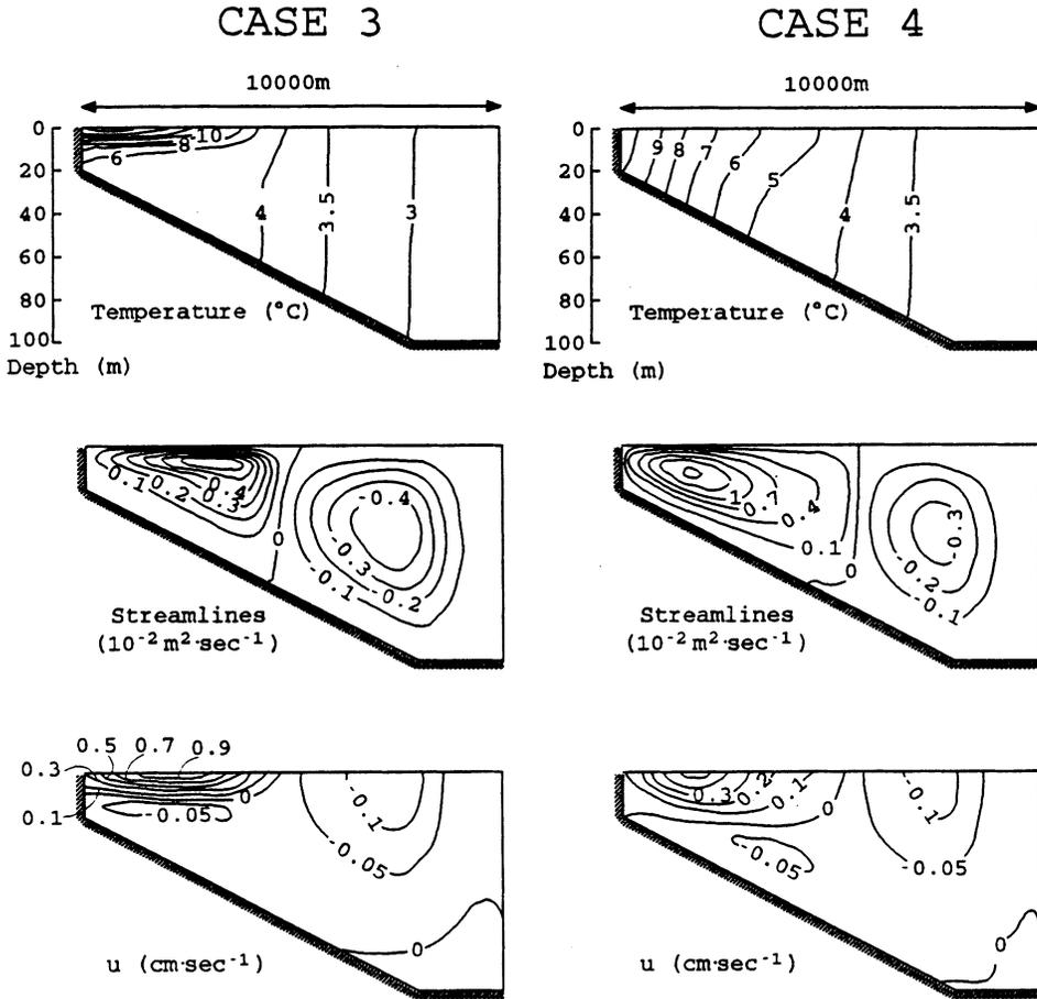
Fig. 3. Obtained temperature distributions, streamfunctions, and long-shore velocity distributions for cases 3 and 4 (section B, with the bottom slope  $10^{-3}$ ) when only density-driven currents were considered. Only half of the cross-section is shown as the center is a symmetry line.
