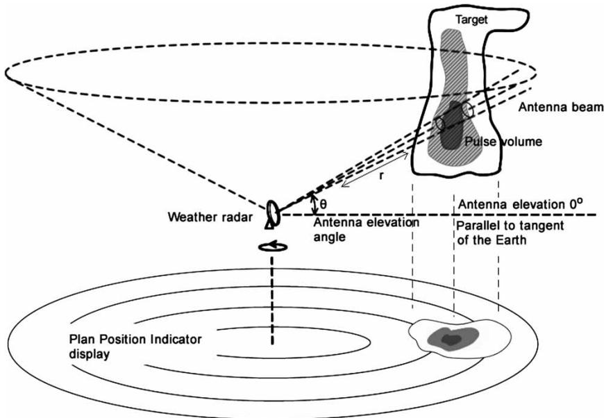
**Figure 1** | Weather radar operation principles producing a plan position indicator (PPI) display.
