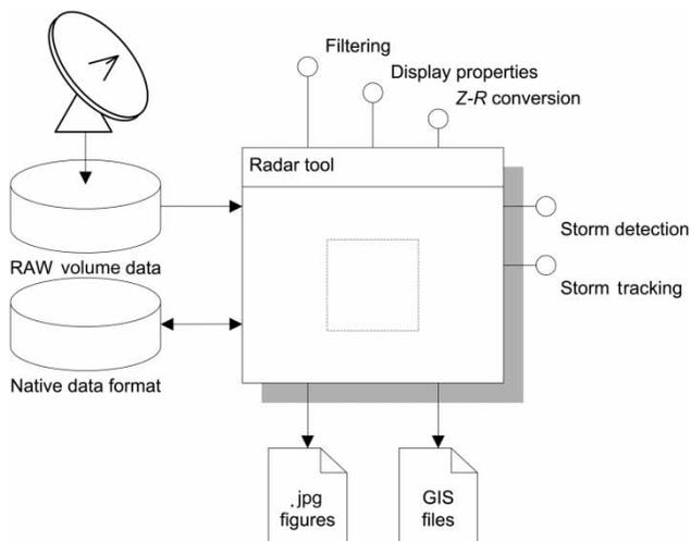
Figure 4 | Weather radar data module features.
