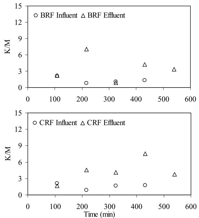
**Figure 8** | Change of influent and effluent sample K/M ratios in unripened calcite and basalt roughing filters.
