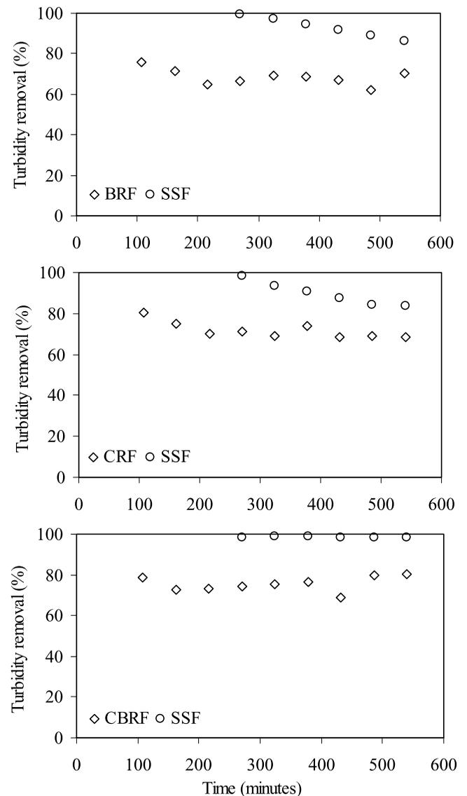
**Figure 5** | Clay turbidity removal of roughing filters and connected slow sand filters during 150 NTU challenge experiments with K-clay to M-clay ratio of 0.3.
