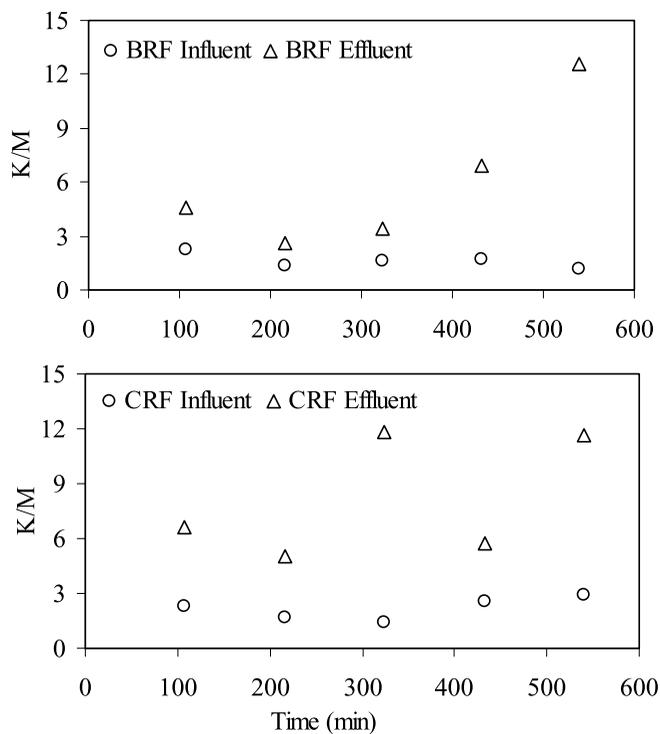
**Figure 9** | Change of influent and effluent sample K/M ratios in ripened calcite and basalt roughing filters.
