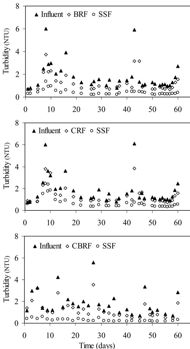
**Figure 4** | Influent and effluent turbidities of the roughing and connected slow sand filters during the 60-day studies.
