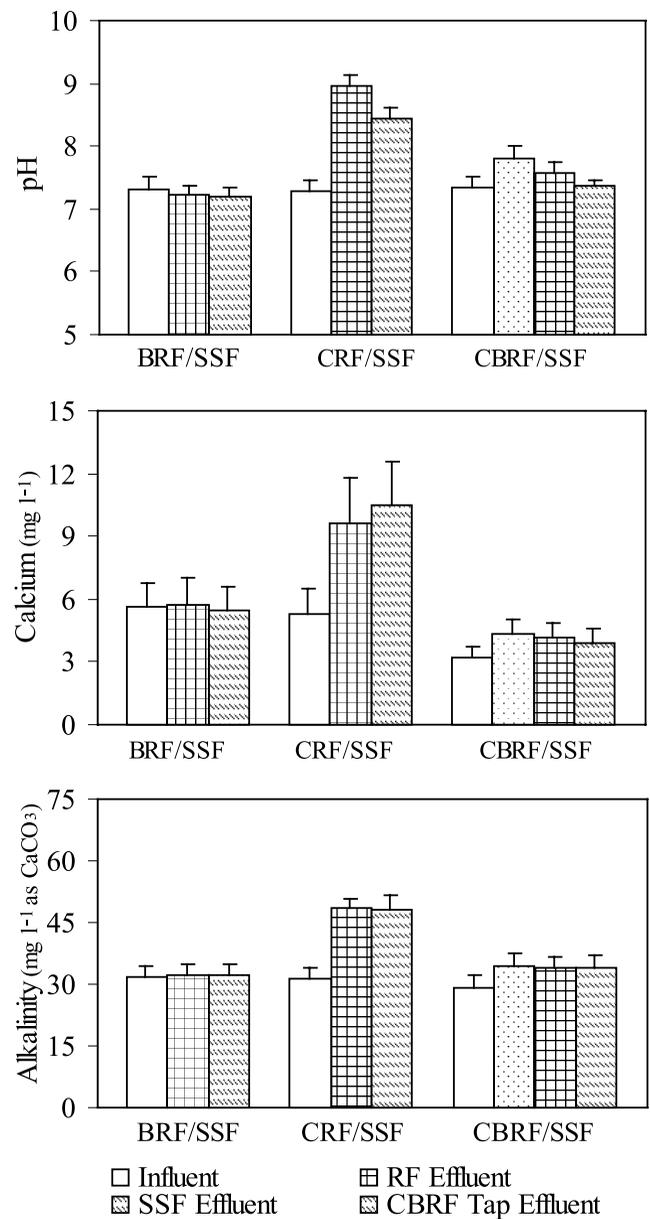
**Figure 2** | pH, calcium and alkalinity results from influent, sample tap and filter effluent grab samples collected during the 60-day filtration studies.
