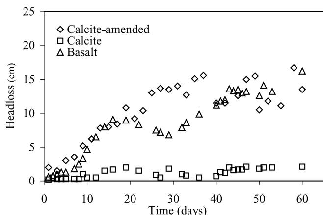
**Figure 3** | Schmutzdecke headloss accumulation of the slow sand filters fed by the calcite, basalt and calcite-amended roughing filters.
