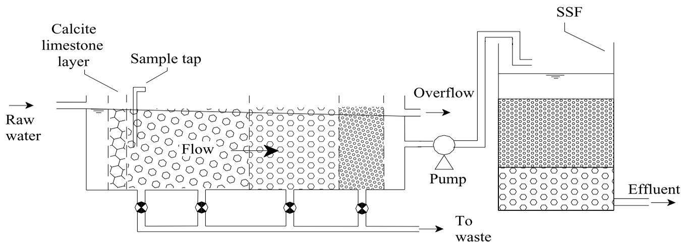
**Figure 1** | Pilot roughing and slow sand filter configuration showing CBRF calcite layer and sample tap. Roughing filter freeboard not shown.
