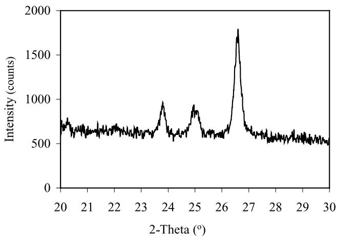
**Figure 6** | X-ray diffraction pattern of Santiam River sample evaporated from 3 l of raw water.
