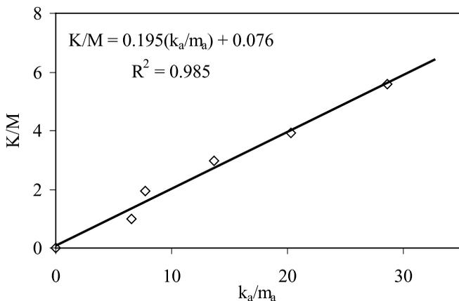
**Figure 7** | Standard curve of XRD-derived K-clay/M-clay peak area ratios ( $k_a/m_a$ ) plotted versus known added clay concentrations (K/M).
