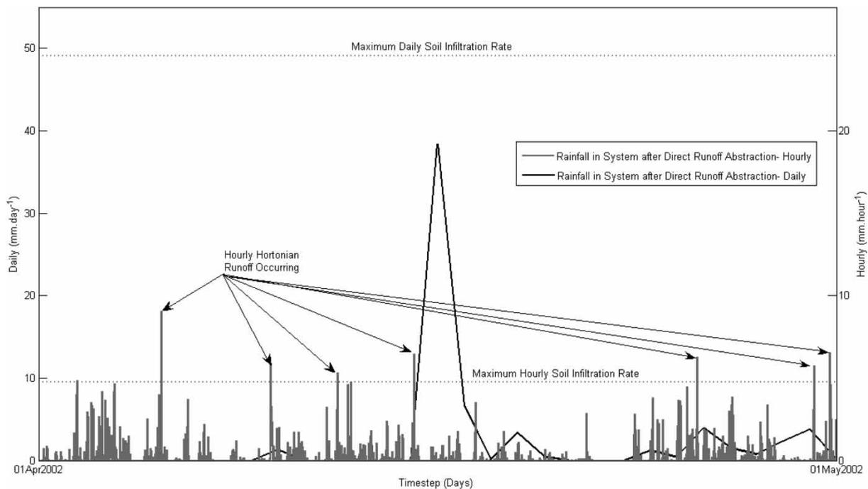
**Figure 7** | Generation of surface runoff via Hortonian runoff pathway,  $r_2$ .
