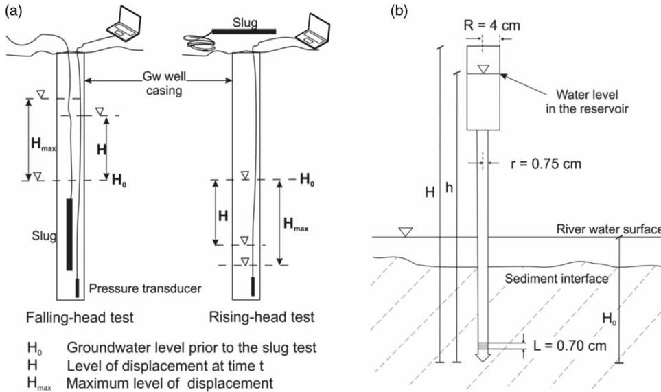
Figure 3 | Devices used for determination of hydraulic conductivity ( $K$ ). (a) Slug test for the aquifer ( $K_{aq}$ ); (b) direct-push piezometer for the clogging layer ( $K_{cl}$ ).
