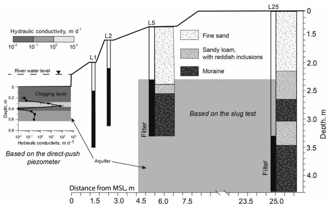
**Figure 5** | Depth profiles of the sediment sequence and mean hydraulic conductivity values along the monitoring transect. Soil profiles based on visual inspection during drilling of L5 and L25 are shown.
