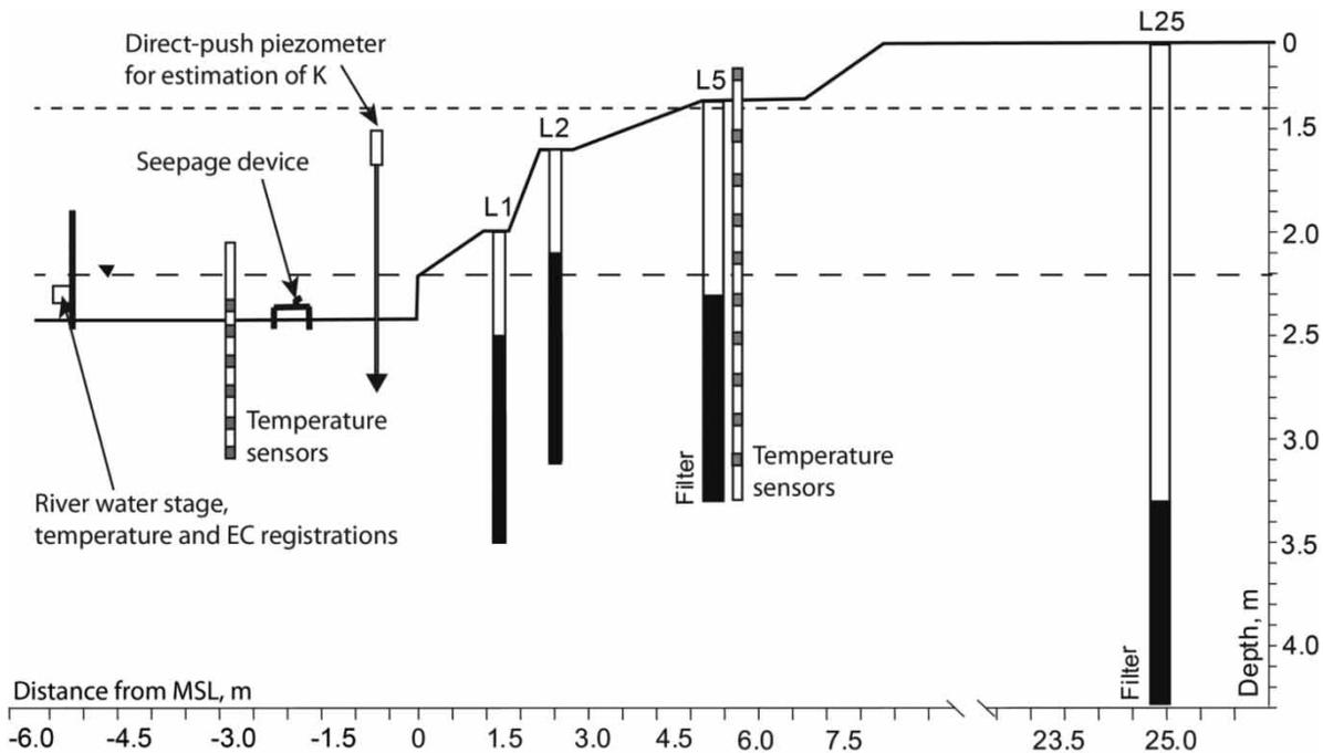
**Figure 2** | Monitoring site for the Lule River. Short dashed line – maximum observed river water and groundwater levels; long dashed line – mean river and groundwater levels; solid line – ground surface. Well number (L1-L25) indicates the distance in metres from the mean shore line (MSL). Sites of temperature profile sensors, seepage meters and direct-push piezometer installations are shown.
