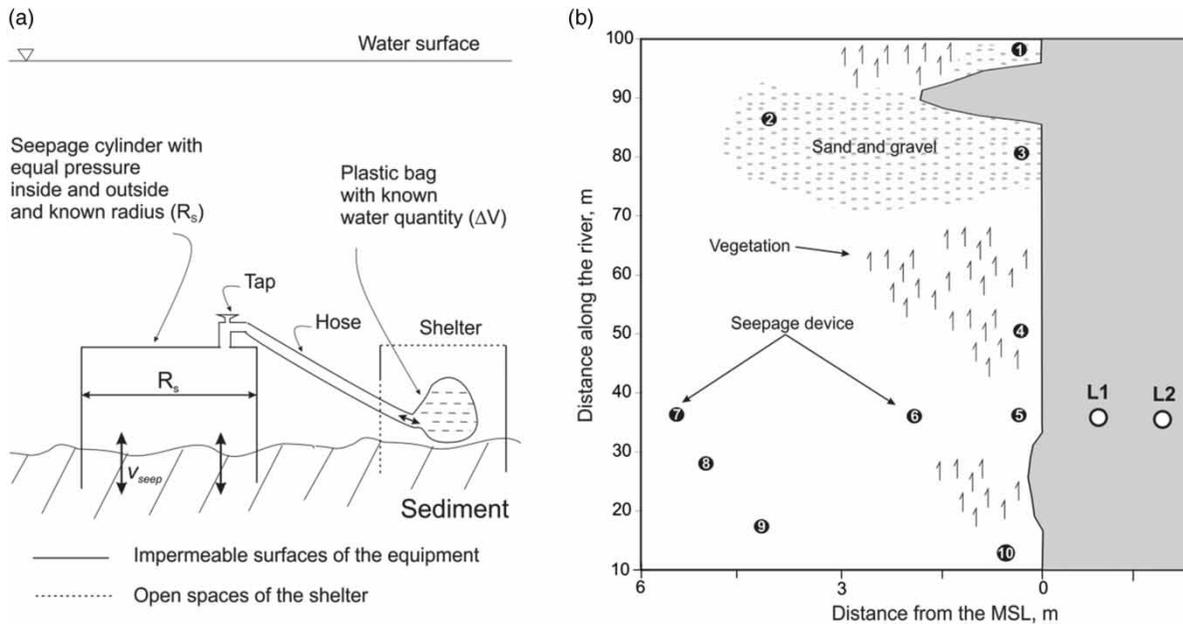
Figure 4 | (a) Device used for assessment of spatial variation in seepage flow and determination of mean equivalent hydraulic conductivity ( $K_E$ ) for the aquifer and the clogging layer; (b) location of the seepage devices and observation wells L1 and L2.
