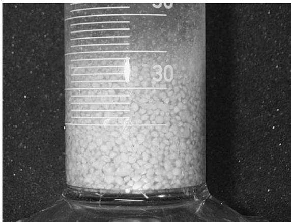
**Figure 5** Granules obtained with synthetic wastewater (organic load = 2.5 kgCOD/m<sup>3</sup>.d)
