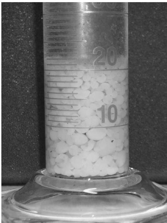
**Figure 7** Granules from industrial wastewater (Load = 3 kgCOD/m<sup>3</sup>.d)
