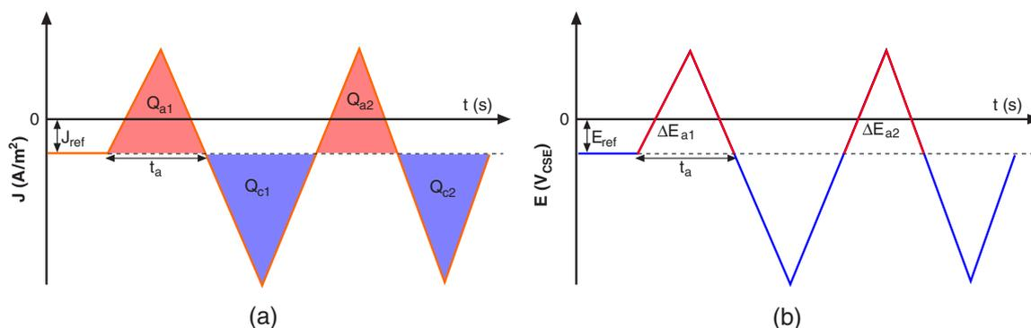
**FIGURE 5.** Schematic evolution of stray current interference of a pipeline for current density in a coating defect or a coupon (a) and pipeline potential (b). The cathodic and anodic charges in (a) are obtained based on the surface integral of the respective current densities. The anodic interference  $\Delta E_{a,avg}$  in (b) is the result of the average anodic shift of the potential relative to  $E_{ref}$ . The duration  $t_a$  corresponds to the longest anodic excursion.
