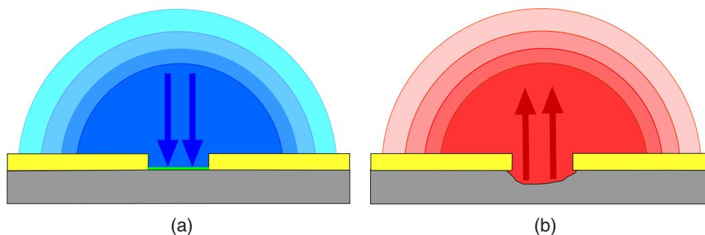
**FIGURE 3.** Schematic illustration of (a) cathodic concentration polarization and (b) anodic concentration polarization. The cathodic current entering the steel surface results in a depletion of oxygen, an increase of the pH value in the soil, and passivation (a). The anodic current leaving the steel surface results in a lowering of the pH value and provokes corrosion (b). The intensity of coloring indicates the extent of pH change.
