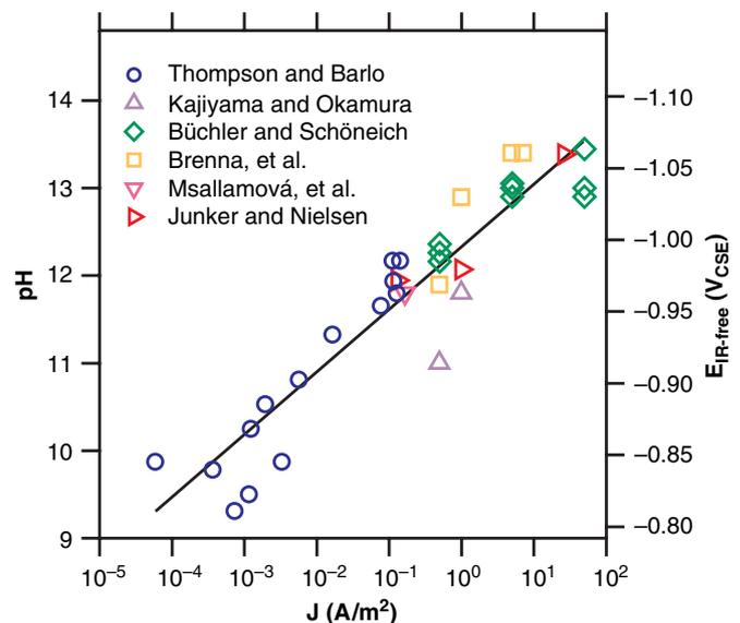
**FIGURE 2.** The pH value at the steel surface as a function of the cathodic current density according to different literature sources summarized in Junker and Nielsen.<sup>17-21</sup> On the right vertical axis, the expected IR-free potentials associated with the hydrogen equilibrium line are shown.
