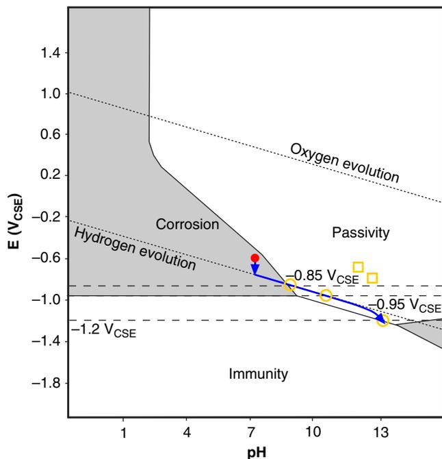
**FIGURE 1.** Pourbaix-diagram (Fe/H<sub>2</sub>O) illustrating the cathodic polarization of steel<sup>15</sup> as a result of activation and concentration polarization. The arrow shows the effect of polarization and the resulting increase of the pH level. The circles and squares indicate the position of the protection potentials according to ISO 15589-1.
