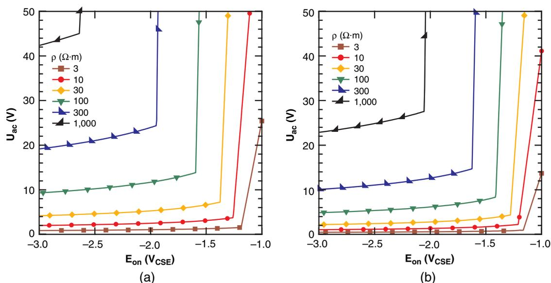
**FIGURE 8.** Admissible average  $U_{ac}$  as a function of the average  $E_{on}$  for various soil resistivities  $\rho$  and an acceptable  $I_{max}$  of 5 mm calculated with the parameters in Büchler and Joos<sup>47-48</sup> for: (a) PE and (b) FBE coatings.
