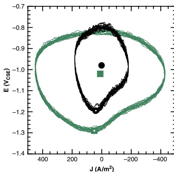
**FIGURE 7.** IR-free potentials determined on ER coupons as a function of the current density ( $J$ ) under AC interference of 16.7 Hz (cathodic currents with a positive sign). Disk symbols: no corrosion at  $J_{dc} 1 A/m^2$ ,  $J_{ac} 128 A/m^2$ . Square symbols: corrosion at  $J_{dc} 11 A/m^2$ ,  $J_{ac} 309 A/m^2$  according to Bette.<sup>43</sup> The full symbols correspond to  $E_{IR-free}$  and the empty symbols to the most negative cathodic excursion called  $E_H$ .
