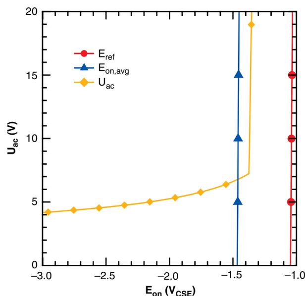
**FIGURE 9.** Admissible average  $U_{ac}$  and average  $E_{on}$  for ensuring effective CP in case of combined DC and AC stray current interference:  $E_{ref}$  required to ensure effective CP with  $J_{ref}$  of 0.1  $A/m^2$  in absence of any interference;  $E_{on,avg}$  for effective corrosion protection in case of anodic DC interference; and  $U_{ac}$  for protection against AC corrosion.
