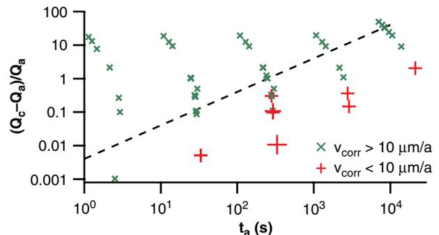
FIGURE 6. Experimental determination of  $Q$  as a function of  $t_a$  in artificial soil and hard water. The dotted line represents the minimum requirement for protection against stray current corrosion, i.e.,  $(|Q_c| - |Q_a|)/|Q_a| = t_a \times 0.004 \text{ s}^{-1}$ .
