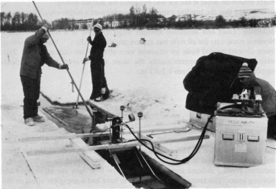
Fig. 1. Schematic of test frame and field installation. Flexural failure precipitated at bottom of ice samples.
