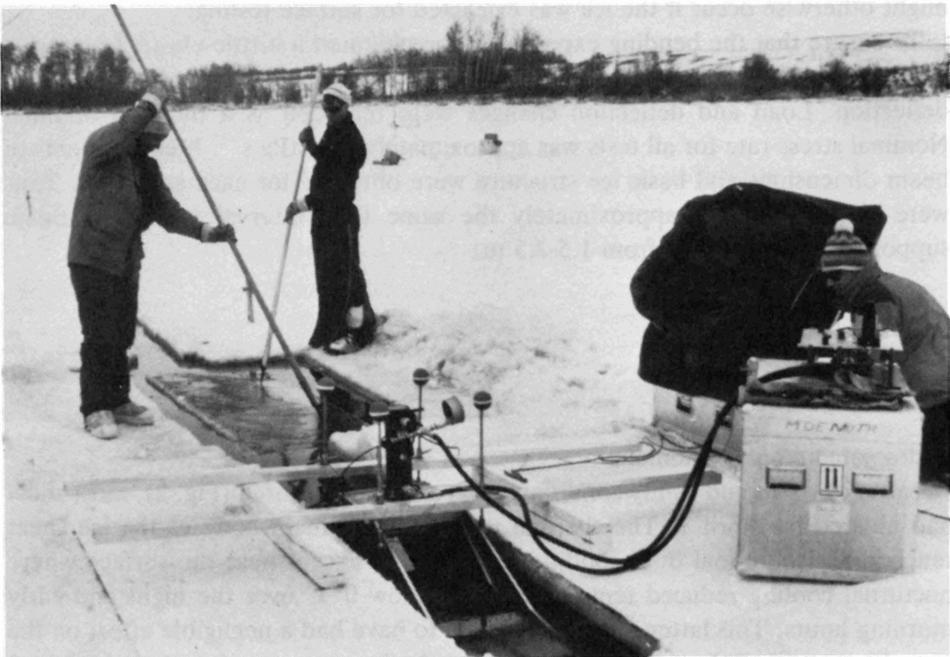
Fig. 1. Schematic of test frame and field installation. Flexural failure precipitated at bottom of ice samples.
