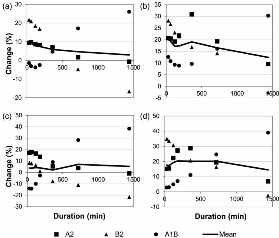
**Figure 7** | Relative changes in 10-year precipitation intensity in projections A2, B2 and A1B (black circles) and mean changes (lines). Top row: tuned downscaling for period FC1 (2011–2040; (a)) and FC3 (2071–2100; (b)). Bottom row: untuned downscaling for period FC1 (c) and FC3 (d).
