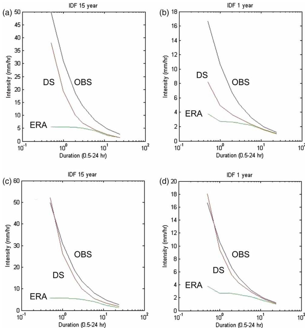
**Figure 5** | IDF curves representing observations (Equation (1); OBS), ERA simulation grid box precipitation (ERA) and point simulations by downscaling (DS). Top row: untuned downscaling for return periods 15 years (a) and 1 year (b). Bottom row: tuned downscaling for return periods 15 years (c) and 1 year (d).
