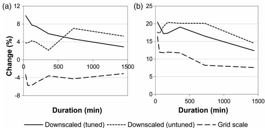
**Figure 8** | Relative change in 10-year precipitation intensity from REF to FC1 (2011–2040; (a)) and FC3 (2071–2100; (b)) estimated by tuned downscaling, untuned downscaling and at the grid box scale. The curves represent averages over the three projections used, i.e. A2, B2 and A1B.
