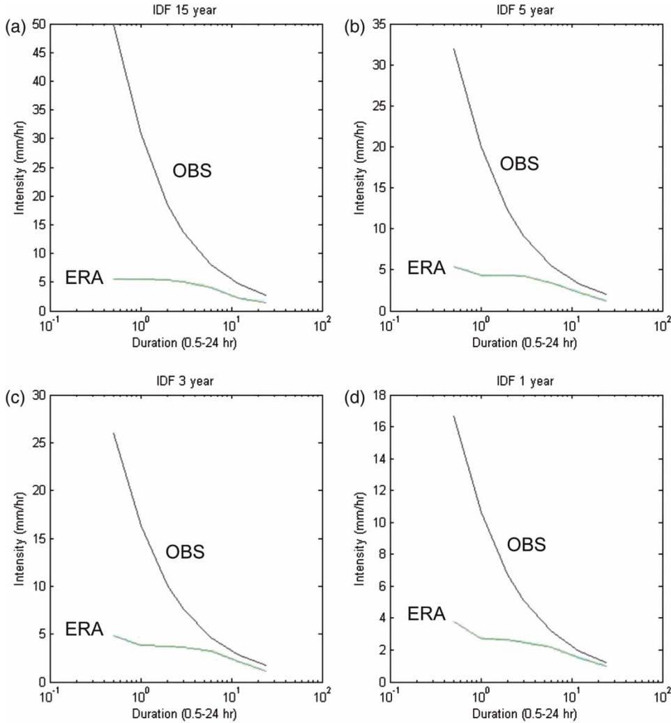
**Figure 3** | IDF curves representing observations (Equation (1); OBS) and ERA simulation grid box output (ERA) for return periods 15 (a), 5 (b), 3 (c) and 1 (d) year(s). Note that different scales are used on the y-axis.
