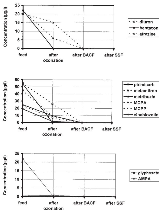
**Figure 11** | Removal of pesticides during a 3-day spiking experiment by ozonation, activated carbon filtration and slow sand filtration in the integrated membrane system.
