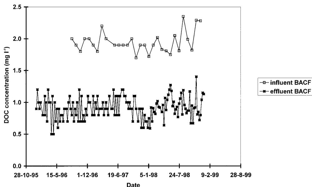
Figure 4 | DOC concentration after biological activated carbon filtration in the full-scale Leiduin plant 1996–1998.
