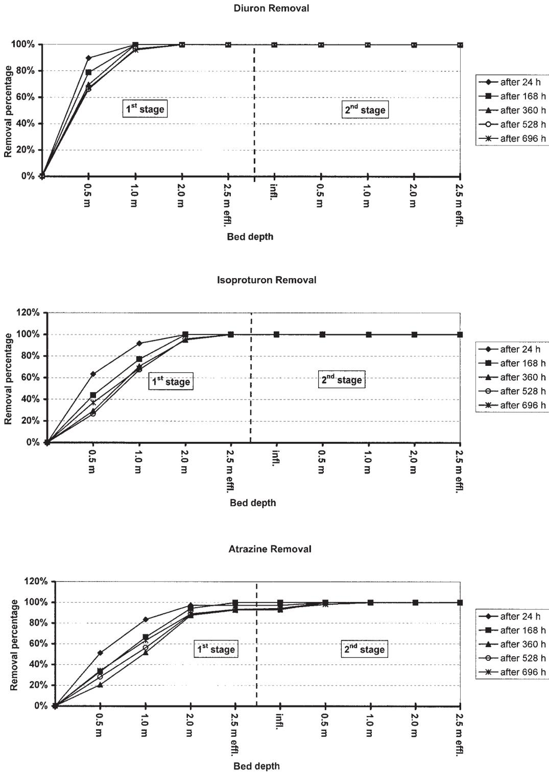
Figure 5 | Removal of diuron, isoproturon and atrazine in a two-stage activated carbon filtration process during a 29-day spiking experiment after a carbon lifetime of 3 years.
