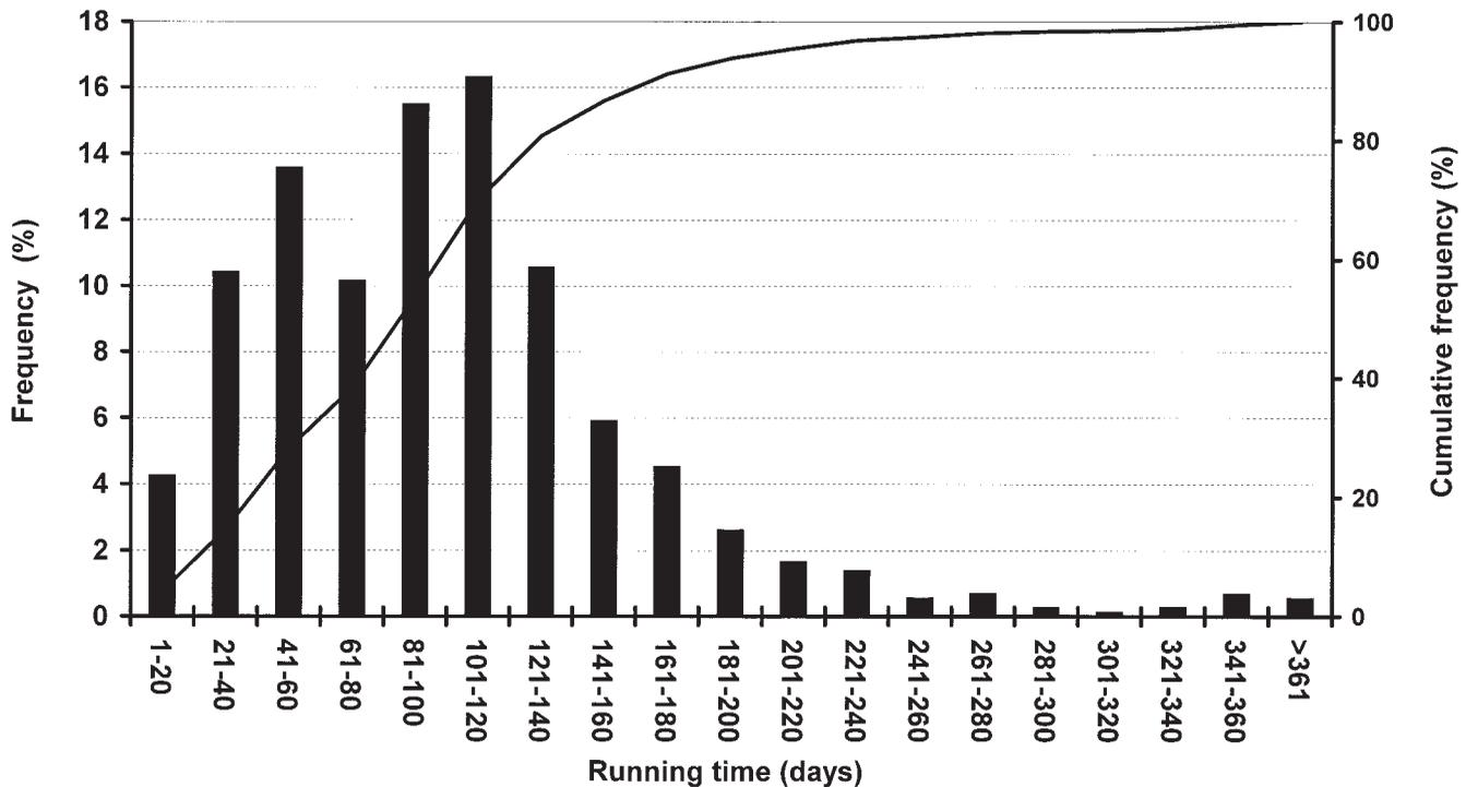
Figure 7 | Running time of the slow sand filters of Leiduyn production plant before the introduction of BACF (1985-1994).
