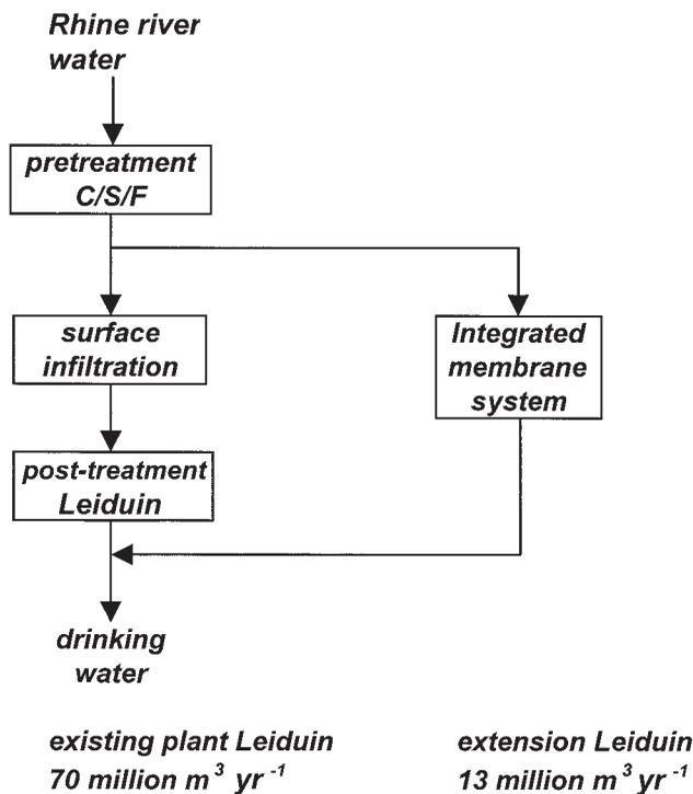
**Figure 9** | Extension of the Leiduin plant with an integrated membrane system.
