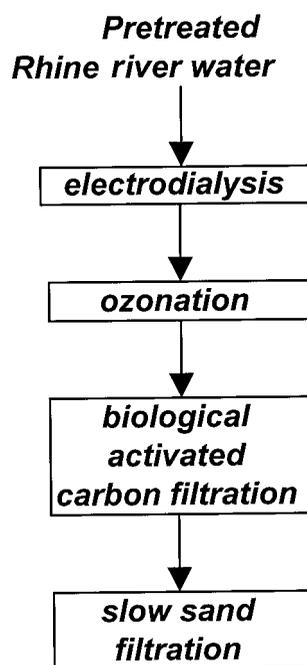
**Figure 13** | An integrated membrane system comprising electro dialysis as alternative for reverse osmosis.
