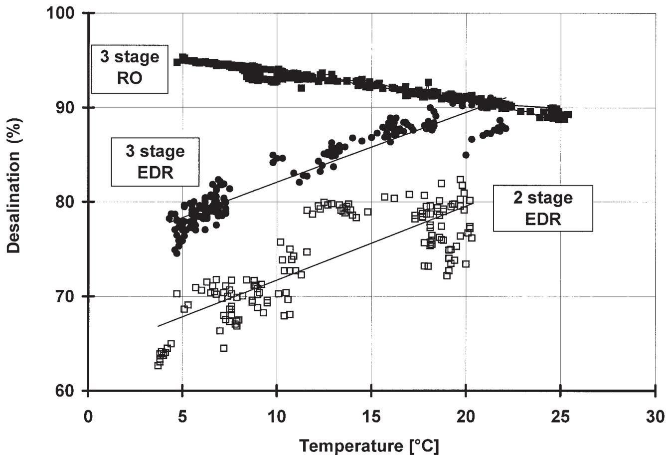
Figure 14 | Desalination characteristics of two stage electro dialysis, three stage electro dialysis, and three stage reverse osmosis.
