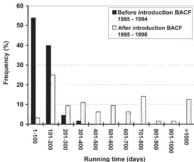
Figure 8 | Running time of the slow sand filters of Leiduyn production plant before and after the introduction of BACF.
