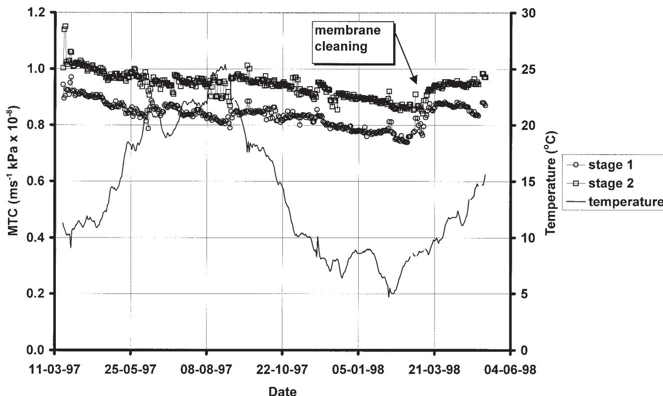
**Figure 10** | Mass transfer coefficient of a reverse osmosis membrane unit, using ozone-activated carbon filtration and slow sand filtration as pretreatment.
