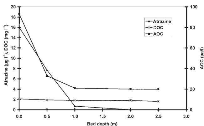
**Figure 6** | Removal of atrazine, DOC and AOC over the filter bed height during a 2-day spiking experiment, using carbon with a lifetime of 36,000 BV (influent DOC 2.1 mg l<sup>-1</sup>; preceding ozone dose 0.8 mg l<sup>-1</sup>).
