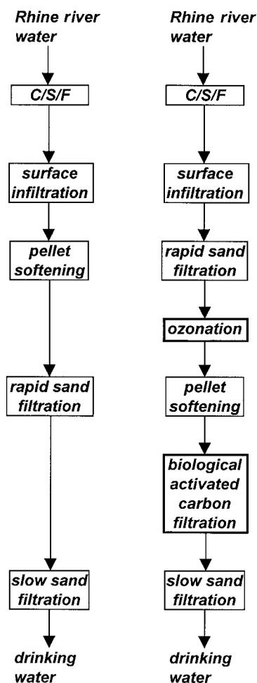
**Figure 1** | Leiduin production plant before (left) and after (right) introduction of BACF.
