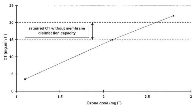
**Figure 12** | Relation between ozone dose and CT value for the pretreated Rhine river water (DOC 2 mg l<sup>-1</sup>; Br<sup>-</sup> 100–200 µg l<sup>-1</sup>).
