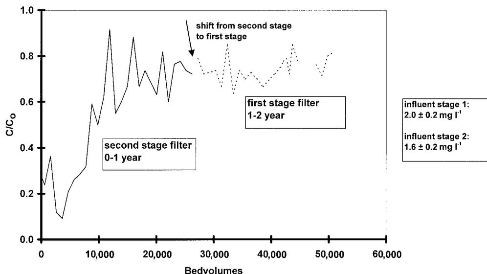
Figure 3 | DOC break-through profile of a single carbon filter in the Leiduin full-scale production plant.
