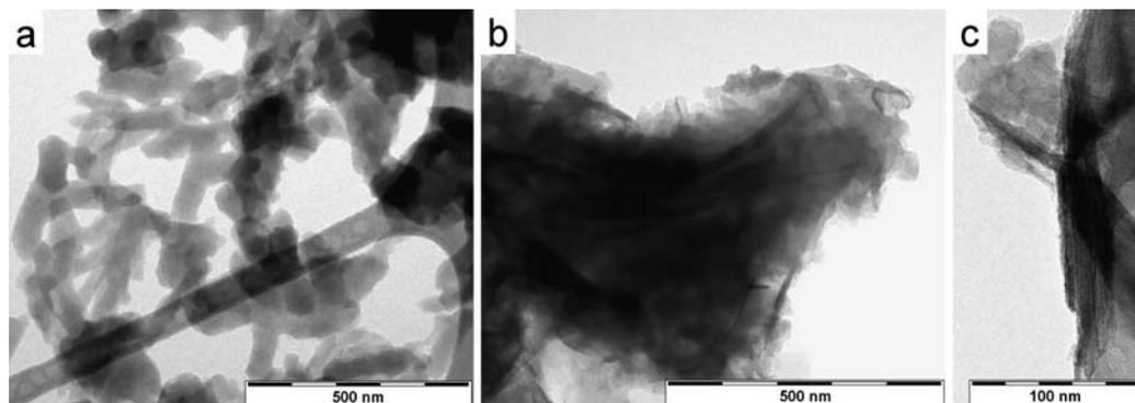
FIG. 6. (a) TEM image of the PANI powder; the sample is composed of rod-shaped grains  $\sim 200$  nm long and diameter of  $\sim 50$  nm. (b) and (c) Covering of the MMT particles (dark elongated bodies) by PANI in the composite.
