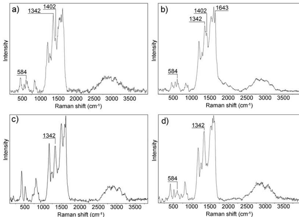
FIG. 7. Raman spectra: (a) of the PANI powder; (b) of the PANI/MMT powder; (c) of the PANI thin film; and (d) of the PANI/MMT thin film.
