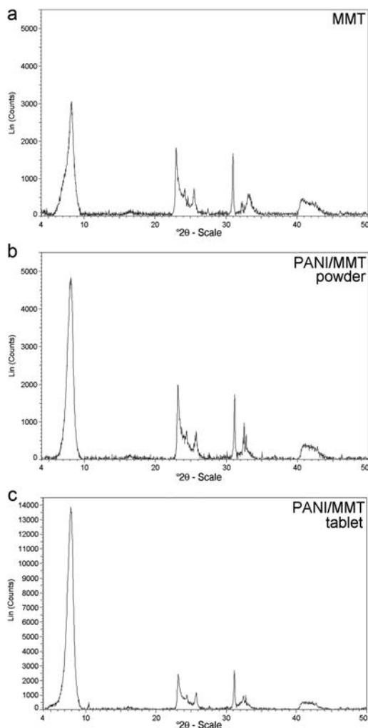
FIG. 4. Full diffraction patterns (range 4–50°2θ) of the MMT powder, the PANI/MMT powder and the PANI/MMT pressed pellet.
