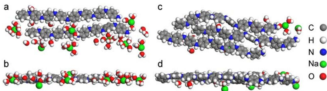
FIG. 5. Optimized models of the PANI/MMT interlayer content showing the interlayer arrangement in the PANI/MMT powder – view along the [001] direction (a); view along the [100] direction (b); and in the PANI/MMT pressed pellet – view along the [001] direction (c); view along the [100] direction (d).
