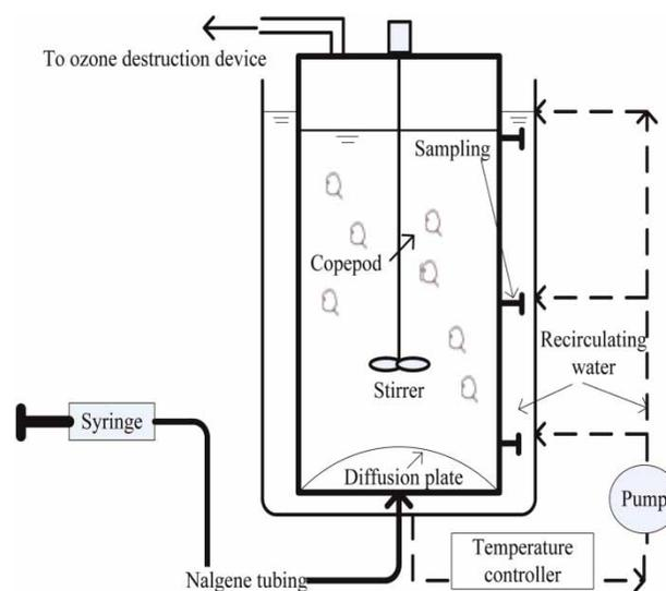
Figure 1 | Scheme of the pilot experiment.
