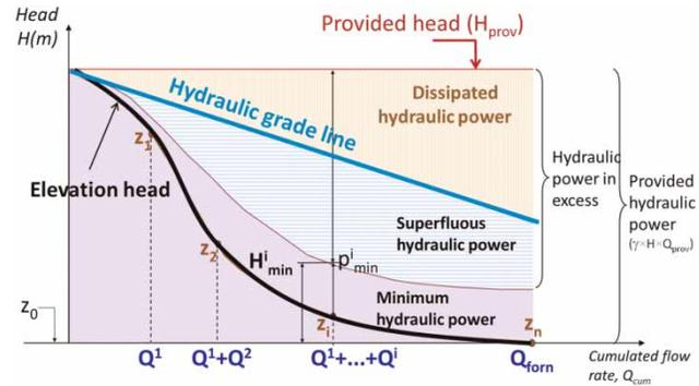
Figure 1 | Schematic representation of the provided power, dissipated power and minimum power.
