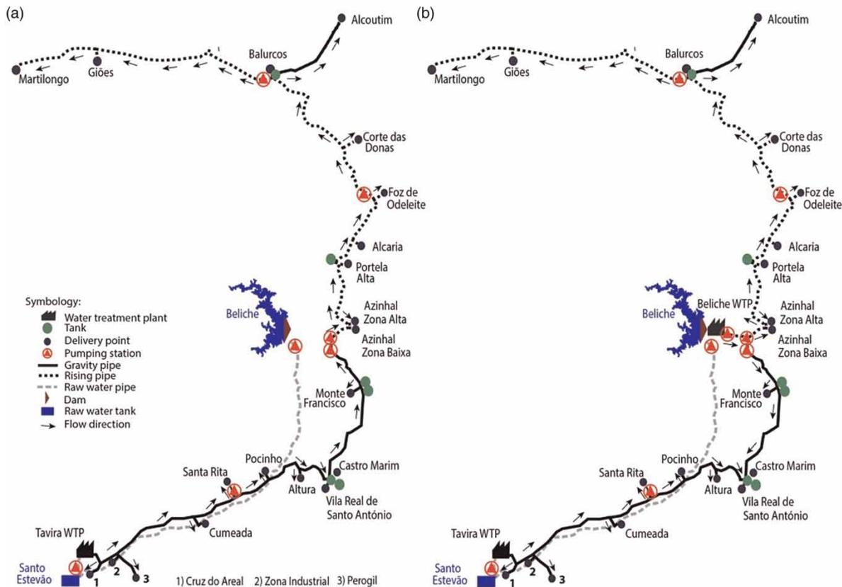
Figure 2 | Operating schemes of the Eastbound system: (a) OS1 and (b) OS2.
