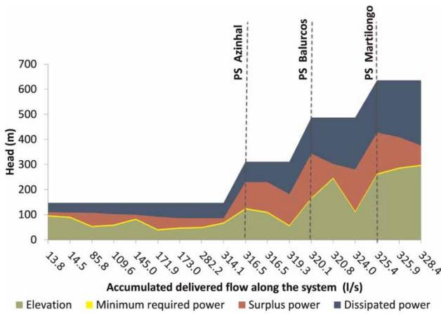
Figure 4 | Minimum, surplus and dissipated power.
