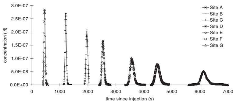
**Figure 3** Concentration profiles from dry weather flow conditions (June 2001)
