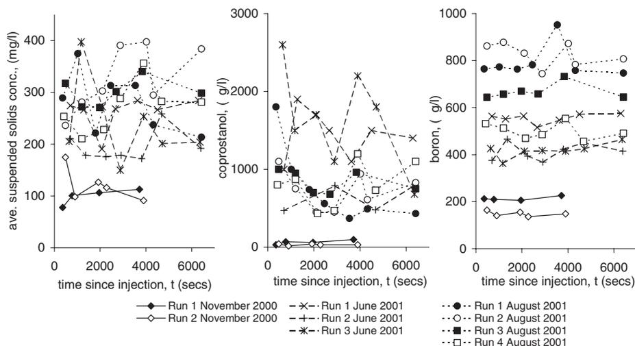
**Figure 4** Suspended solids, coprostanol and boron concentrations versus sample time for all tests and repeats
