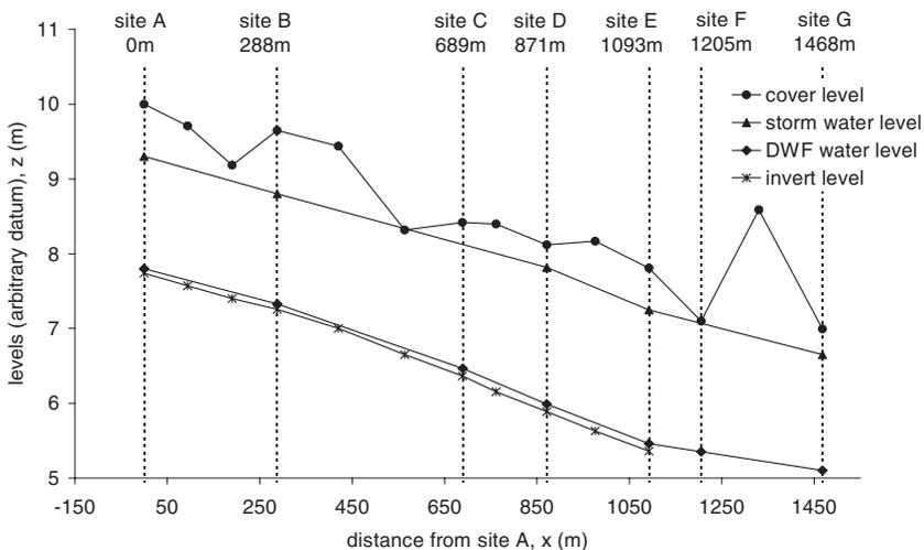
**Figure 1** Longitudinal section of sewer system showing sampling points, levels and surcharge levels, injection was at -150 m
