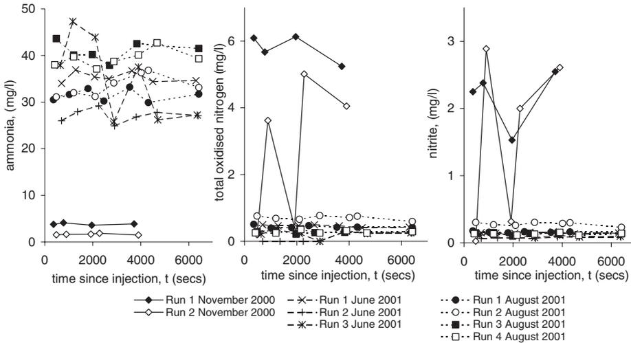
**Figure 5** Ammonia, total oxidised nitrogen and nitrite concentrations versus sample time for all tests and repeats
