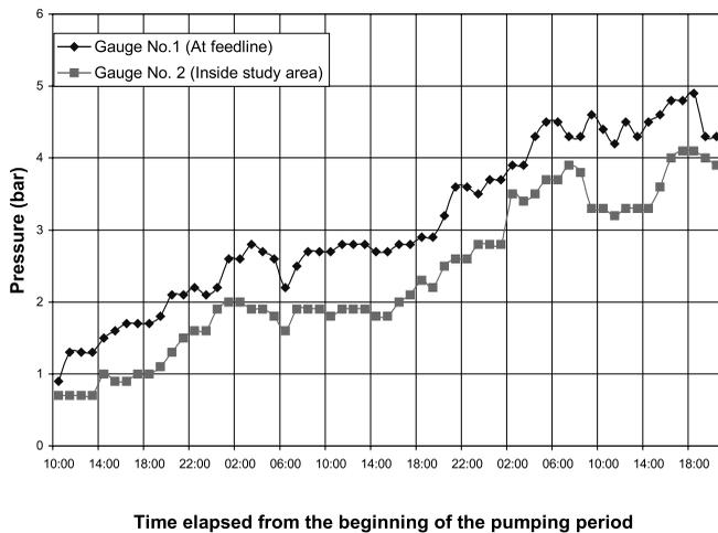
Figure 2 | Pressure variation in study area 4 during pumping period.
