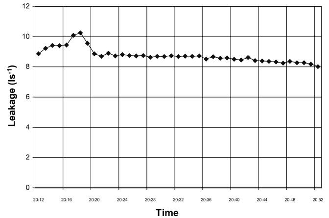
Figure 3 | Leakage in study area 4 during pressure test.
