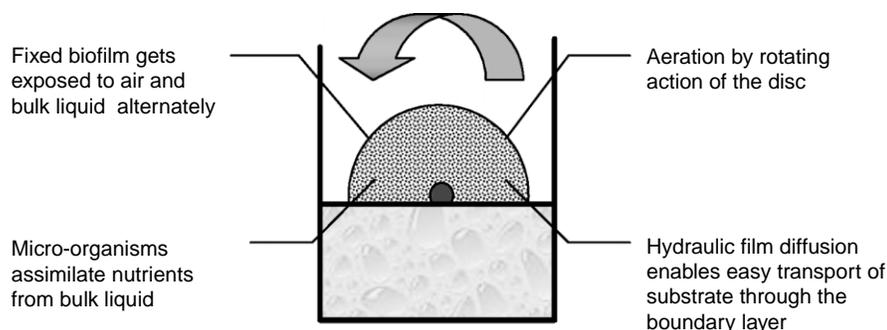
**Figure 1** Sketch of RBC disc with liquid film and biofilm in operation
