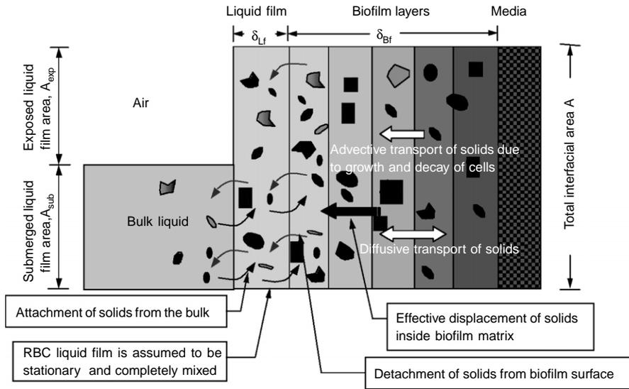
**Figure 2** Transport and detachment of solids occurring in a RBC biofilm
