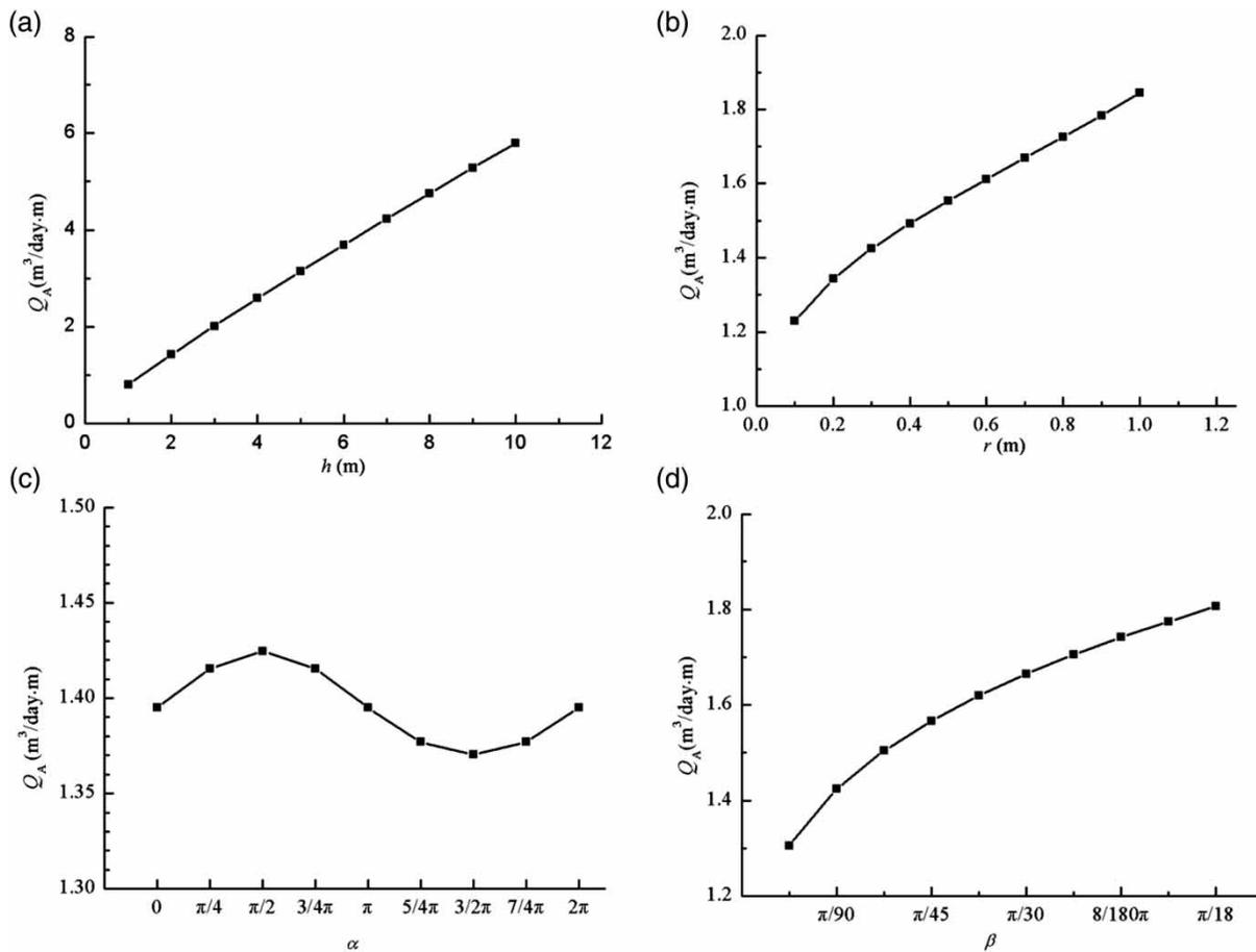
**Figure 3** | Parametric studies. (a) Influence of the hydraulic head; (b) influence of the sewer pipe size; (c) influence of position of the defect; (d) influence of the open size of the defect.
