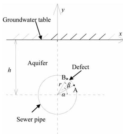
Figure 1 | Sectional view of a sewer pipe with a line defect embedded in semi-infinite aquifer.
