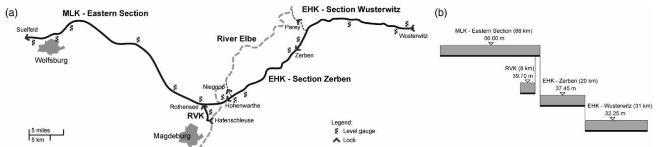
Figure 1 | (a) General map of the navigation canal system Mittellandkanal (MLK)/Elbe-Havel-Kanal (EHK) and (b) elevation of its sections.
