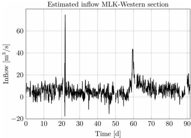
**Figure 7** | Offline estimation of the inflow into the western reach of the MLK between 01 August 2007 and 31 October 2007, see Linke (2007). The gaps indicate failures of the state estimation procedure due to insufficient or erroneous measurements.
