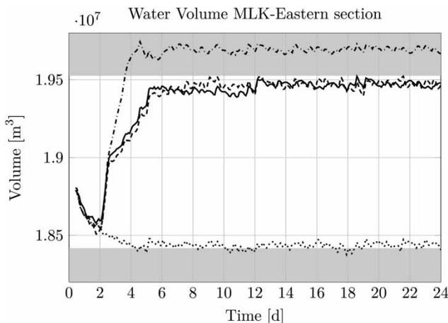
**Figure 9** | Water volume in the MLK-Eastern section. Dotted line is 'w/o additional lateral inflow'; dash-dotted line is 'w/ additional inflow'; solid line is 'w/ additional inflow and prediction'; dashed line is 'w/ additional inflow and prediction, model errors'.
