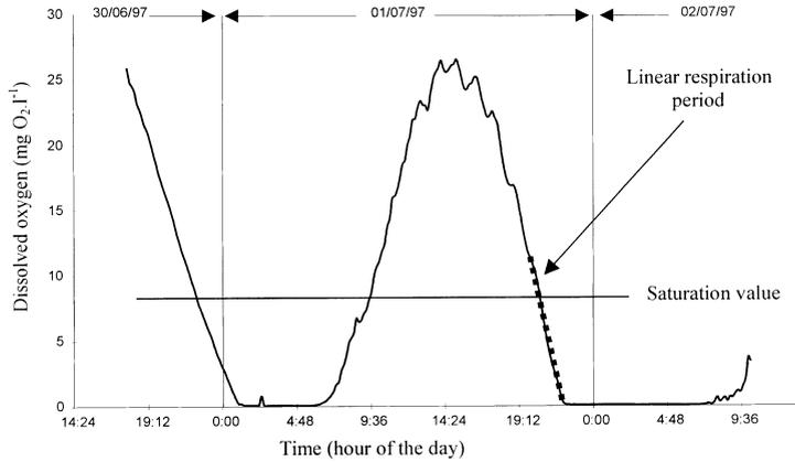
Figure 4 Dissolved oxygen concentration measured in the HRAP
