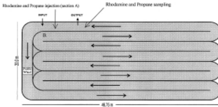
**Figure 1** Diagram of the HRAP located in Rabat
