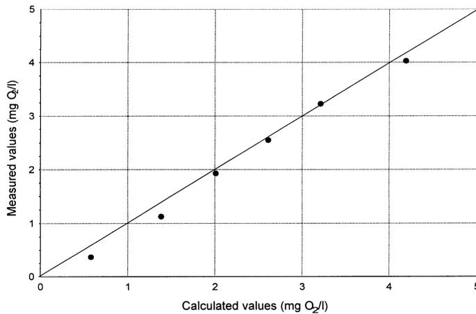
Figure 5 Comparison between observed and calculated  $C_t$
