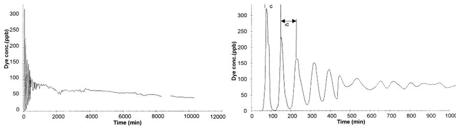
**Figure 2** Tracer response curve after pulse injection (Rabat)
