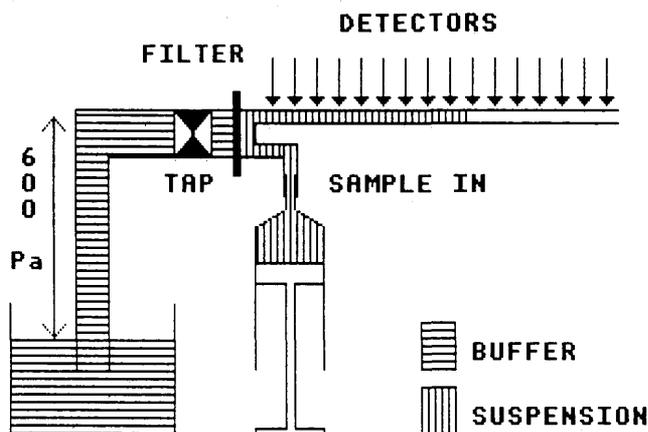
FIG. 1. Schematic drawing of filtration apparatus. Tubing to left of filter is filled with buffer. Pressure head can be adjusted by controlling liquid level in dish. Tubing to right of filter contains suspension, added from syringe, to be filtered. Filtration is started by opening tap. Filtration rate is measured by meniscus passing 39 photodiodes along horizontal tube (arrows).
