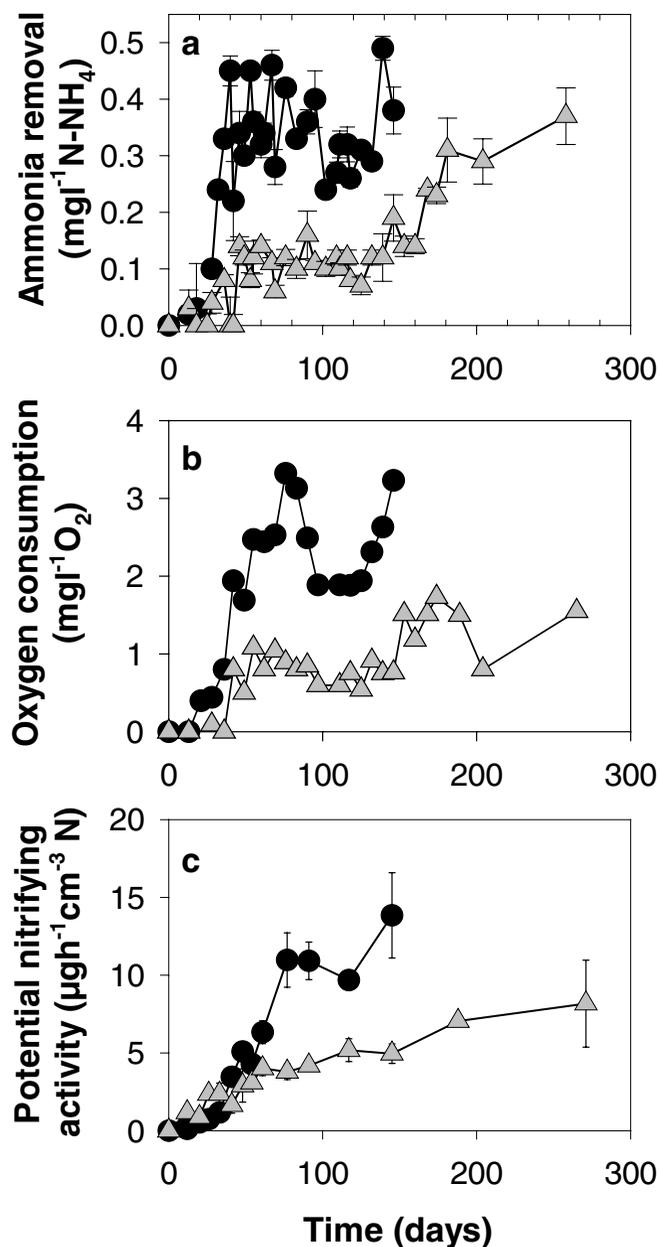
**Figure 1** | Comparison of the ammonia removal (a), the oxygen consumption (b) and the potential nitrifying activity (PNA) in the surface layer (c) in the pilot filtration columns filled with Picabiol (•) and Picacarb ( $\Delta$ ). These filtration columns were fed with settled water enriched with  $0.4 \text{ mg l}^{-1} \text{ N-NH}_4$  at  $20^\circ\text{C}$ . The EBCT in the pilots decreased during the course of the study due to GAC sampling for PNA measurements.
