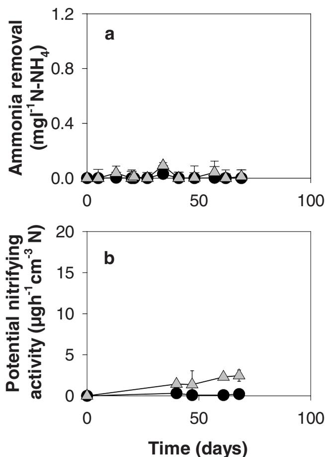
**Figure 3** | Comparison of the ammonia removal (a) and the potential nitrifying activity (PNA) in the surface layer (b) in the pilot filtration columns filled with Picabiol (●) and Picacarb (△). These filtration columns were fed with settled water enriched with 1.2 mg l<sup>-1</sup> N-NH<sub>4</sub> at low temperatures (<7°C). The EBCT in the pilots decreased during the course of the study due to GAC sampling for PNA measurements.
