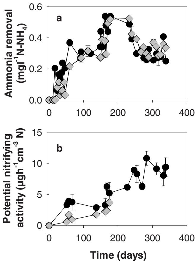
**Figure 4** | Comparison of the ammonia removal (a) and the potential nitrifying activity (PNA) in the surface layer (b) in the pilot filtration columns filled with Picabiol (●) and Calgon F400 (◊). These filtration columns were fed with settled water enriched with  $0.4 \text{ mg l}^{-1} \text{ N-NH}_4$  at  $20^\circ\text{C}$ .
