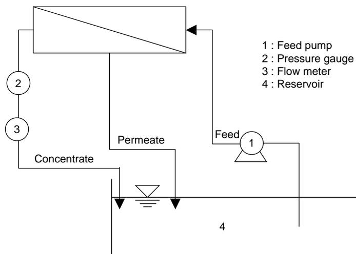
**Figure 2** Cross-flow unit for the adhesion test
