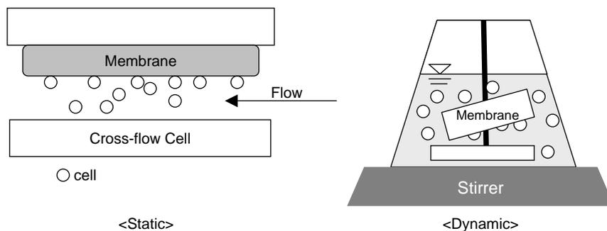
Figure 1 Type of adhesion test
