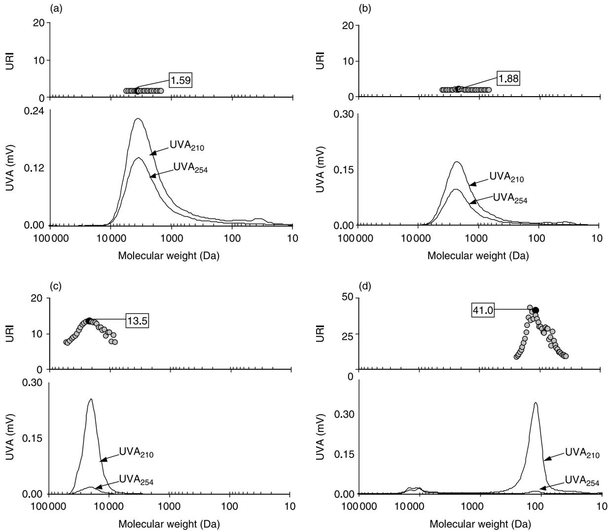
**Figure 5** | Comparison of URI values and HPSEC-UVA chromatograms obtained at 210 nm and 254 nm: (a) SRHA, (b) SRFA, (c) BSA and (d) asparagine.
