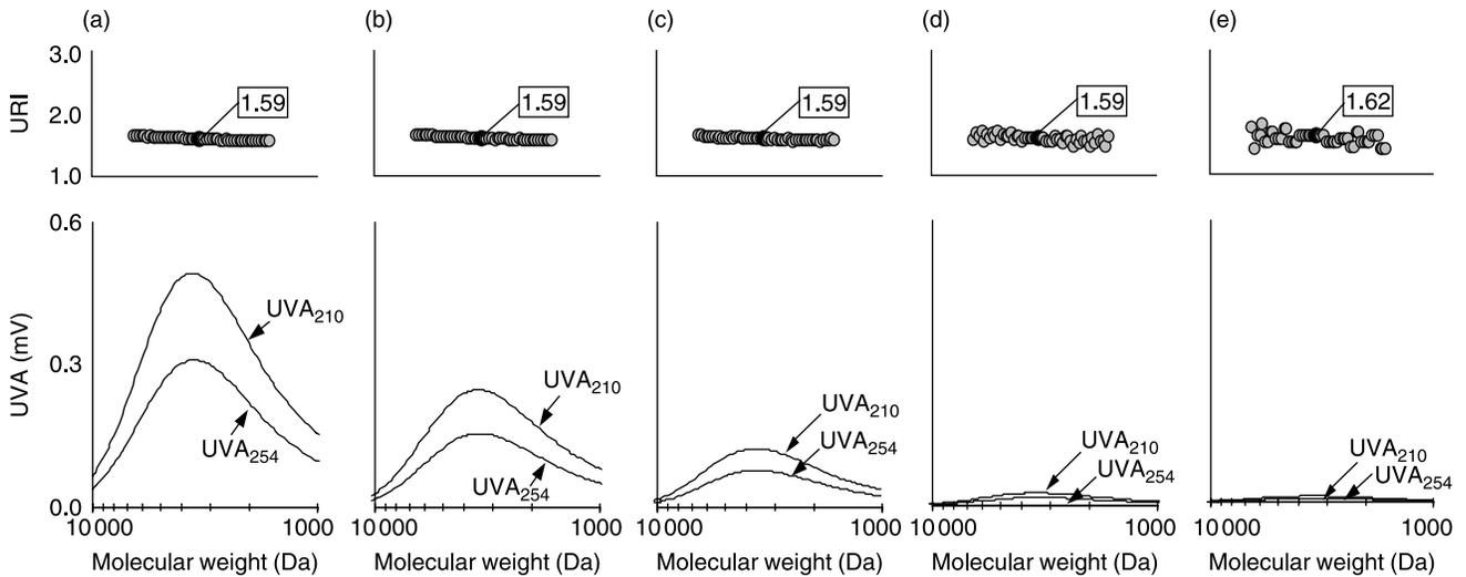
**Figure 2** | Comparison of URI values at different concentrations of SRHA: (a) 20 mg C l<sup>-1</sup>, (b) 10 mg C l<sup>-1</sup>, (c) 5 mg C l<sup>-1</sup>, (d) 1 mg C l<sup>-1</sup> and (e) 0.5 mg C l<sup>-1</sup>.
