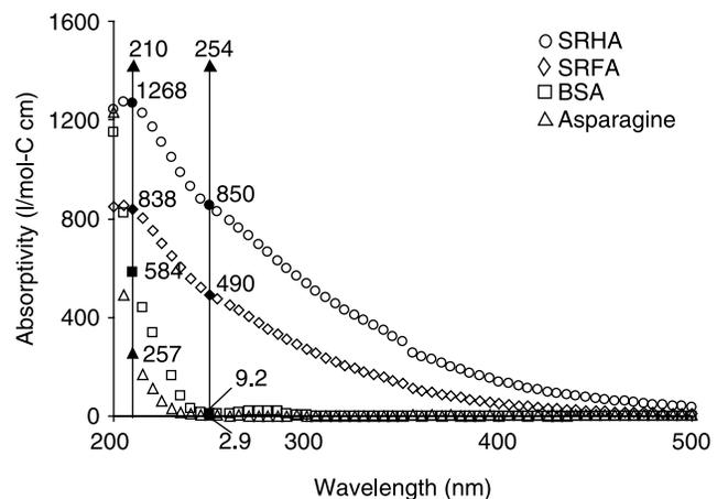
**Figure 4** | Absorptivities based on 1 mol l<sup>-1</sup> of organic carbon for SRHA, SRFA, BSA and asparagine in pure water (pH 7) as a function of wavelength.
