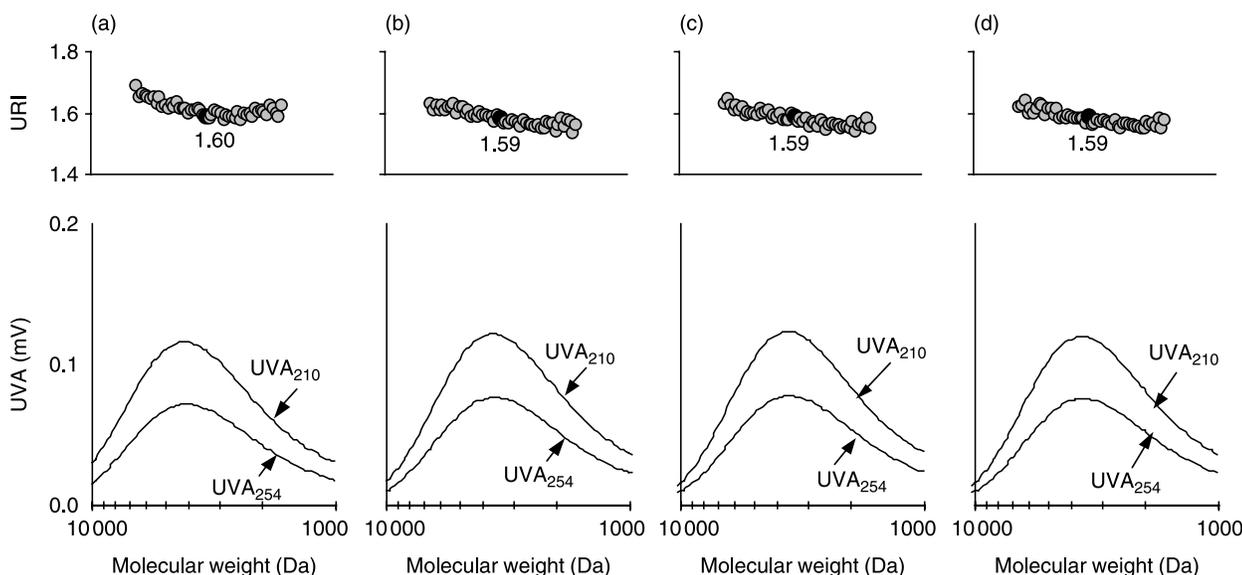
Figure 1 | Reproducibility of both UVA and URI chromatograms (four injections of SRHA of  $5 \text{ mg C l}^{-1}$ ) (numerical value corresponds to peak maximum).
