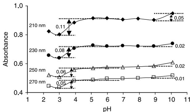
**Figure 3** | UV absorbance of SRHA (10 mg l<sup>-1</sup> as DOC) at different pH conditions (in MQ) for 210 nm, 230 nm, 250 nm and 270 nm.
