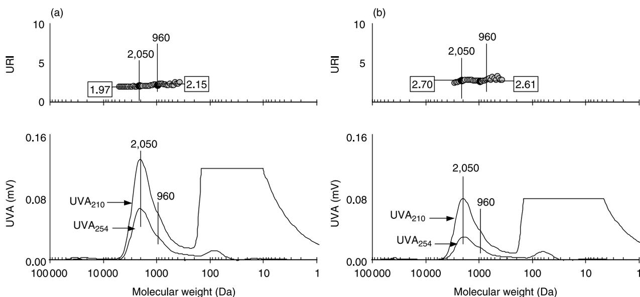
Figure 7 | URI and HPSEC-UVA chromatograms: (a) sand filtered and (b) sand filtered/ozonated Oise River water.
