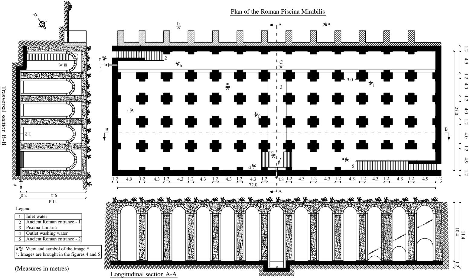
Figure 3 | Plan and sections of the Piscina Mirabilis.
