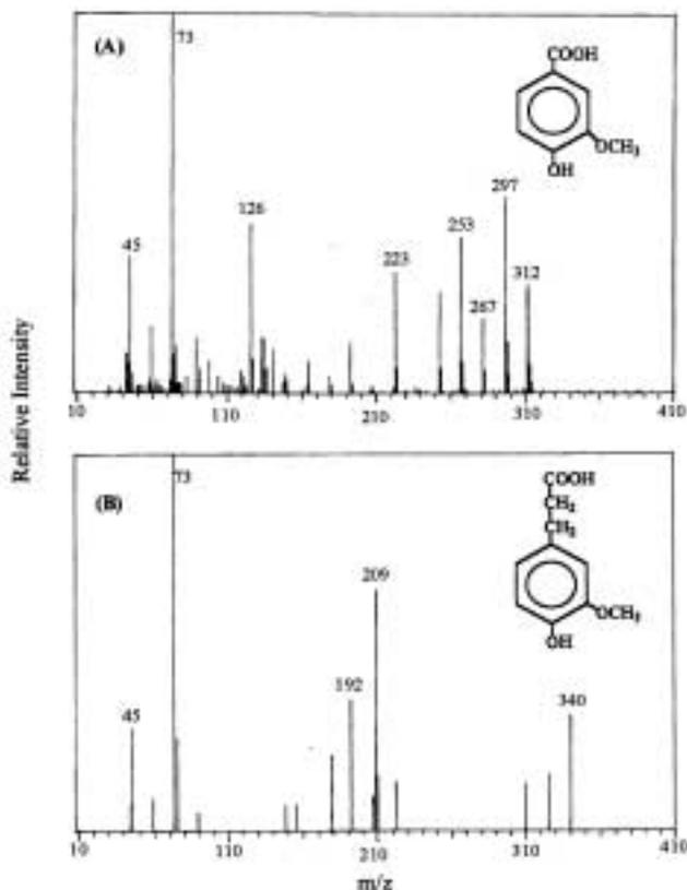
**Figure 5** Degradation by-products of lignin model compound under sulfate reducing condition (A) vanillic acid (B) 3-methoxy-4-hydroxy benzene propionic acid
