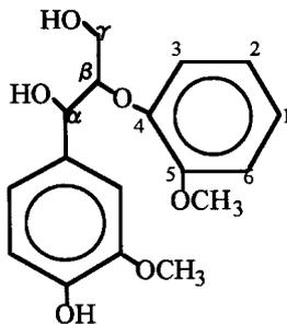
**Figure 1** Lignin model compound with  $\beta$ -O-4 link
