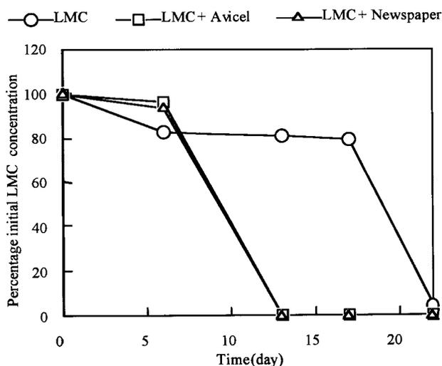
**Figure 4** Degradation of lignin model compound (LMC) with ( $\square$  &  $\triangle$ ) and without ( $\circ$ ) additional source of carbon
