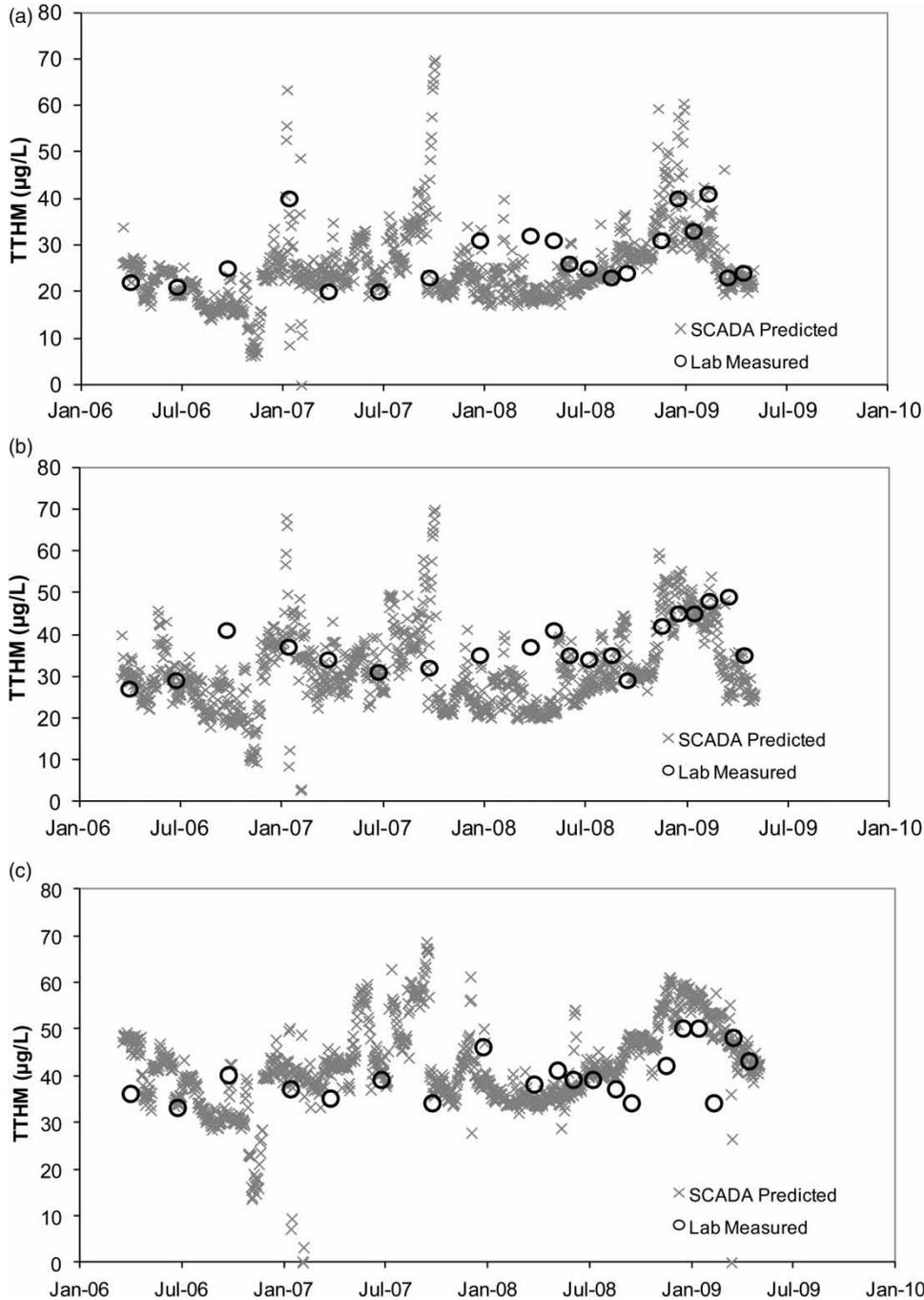
**Figure 7** | TTHM comparison at three turnout locations in the distribution system: (a) AMS-4, (b) AMS-5, and (c) AMS-6.
