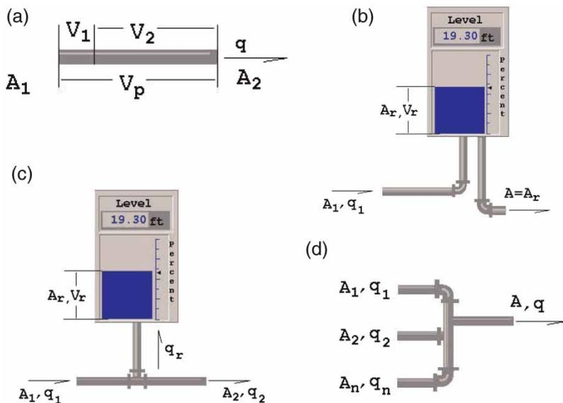
**Figure 2** | Hydraulic model flow conditions: (a) pipe segment, (b) water age for a reservoir, where all flow goes through the reservoir, (c) water age for a reservoir, where net flow is calculated to the reservoir, and (d) water age for two or more streams being mixed.
