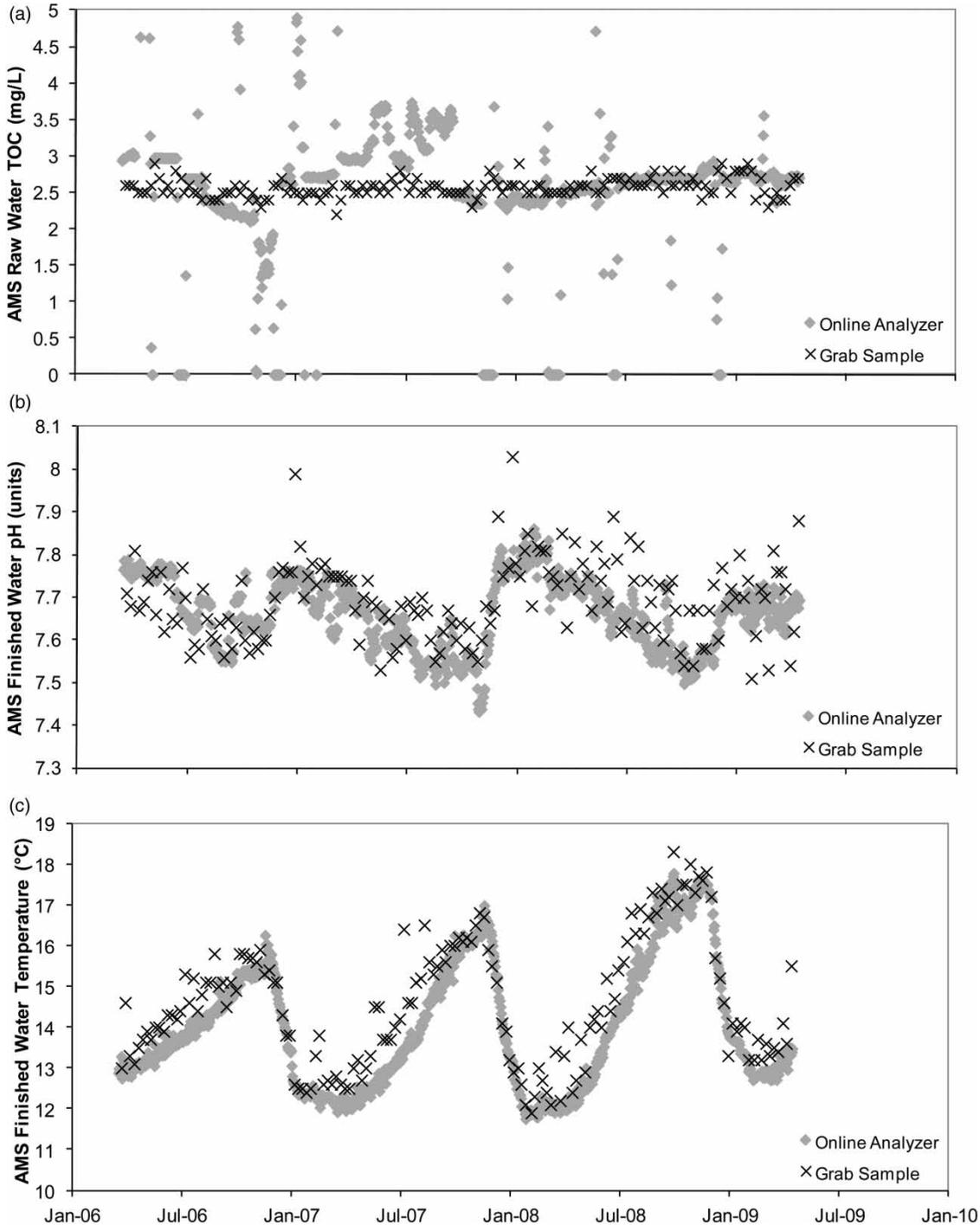
**Figure 4** | Comparison of daily average online water quality instrumentation and weekly grab sample analysis: (a) TOC, (b) pH, and (c) temperature.
