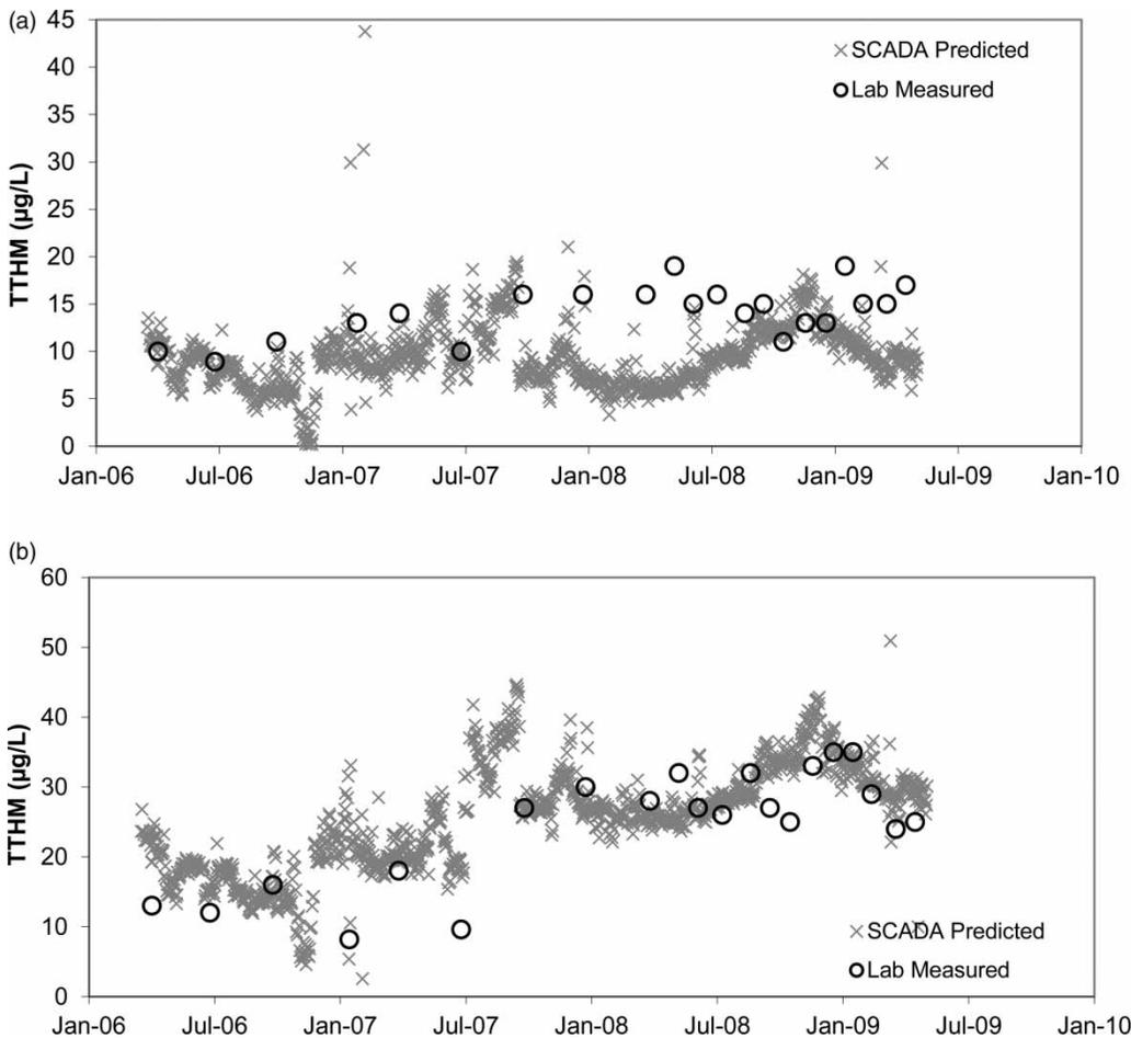
**Figure 6** | TTHM comparison in the finished water at both water treatment facilities: (a) AMS-1 and (b) RM-1 (Note: Prechlorination began in July 2007 for the control of quagga mussels at site RM-1).
