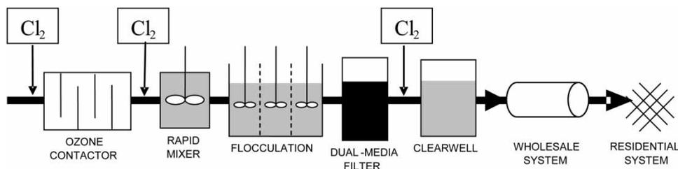
Figure 1 | Schematic of the drinking water treatment and transmission processes with chlorine application points identified.
