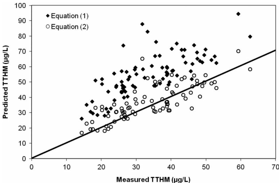
Figure 3 | Comparison of predicted and measured TTHM values using Equations (1) and (2). (Note: Line of equality shown for reference.)
