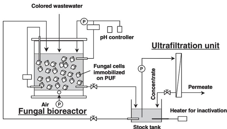
**Figure 1** Schematic diagram of sequencing batch fungal/UF system for decolorization of colored wastewater
