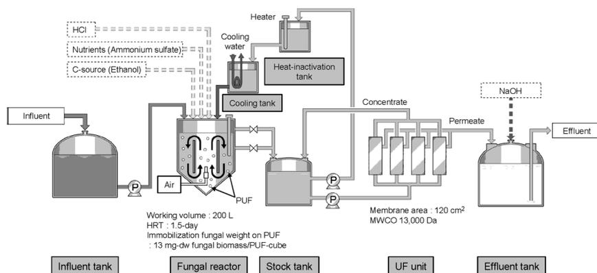
**Figure 4** The schematic diagram of the pilot-scale fungal/UF system for decolorization of colored wastewater
