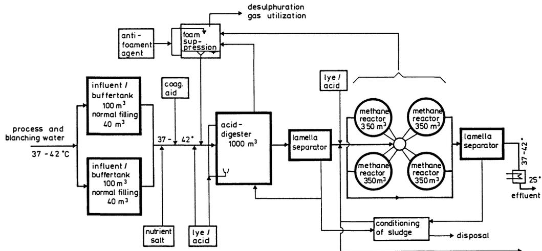
Fig. 5. Flow diagram of the anaerobic wastewater treatment plant of a potato-starch factory (KWU)
