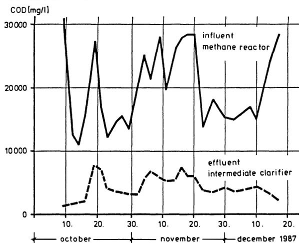
Fig. 2. Operating results for the molasses distillery fixed-film anaerobic digester
