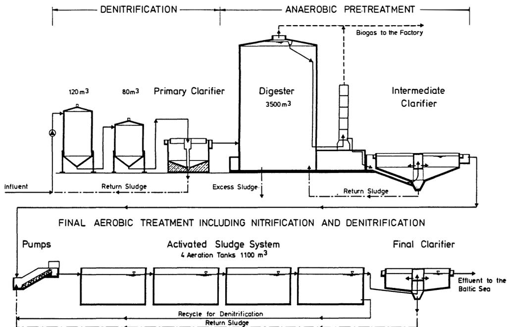
Fig. 7. Flow diagram of the pectin factory anaerobic/aerobic wastewater treatment plant
