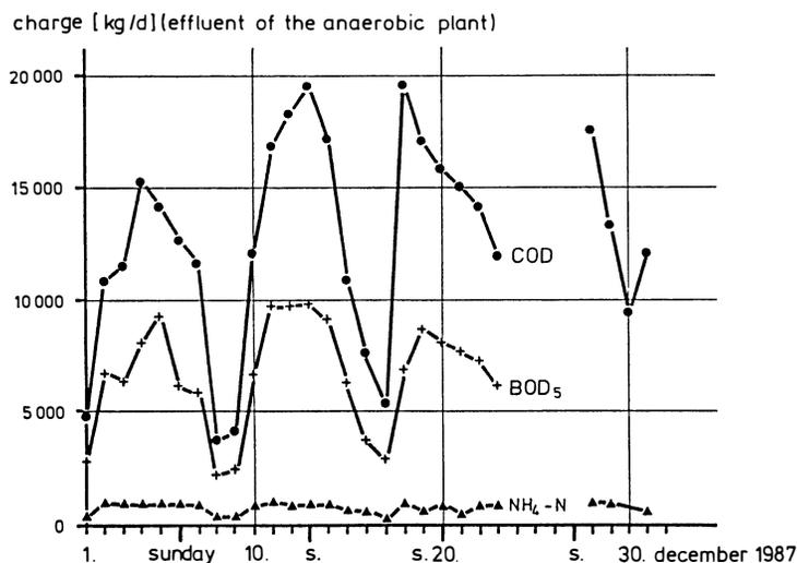
Fig. 6. Operating results (effluent load) of the anaerobic wastewater treatment plant of a potato-starch factory
