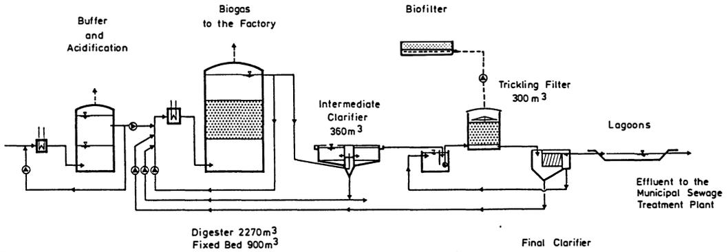
Fig. 3. Flow diagram of the wheat-starch factory anaerobic/aerobic wastewater treatment plant
