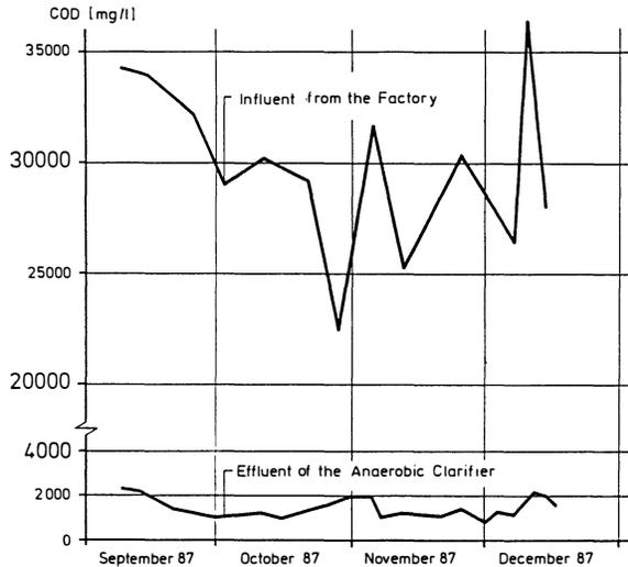
Fig. 4. Operating results of the anaerobic plant of a wheat-starch factory
