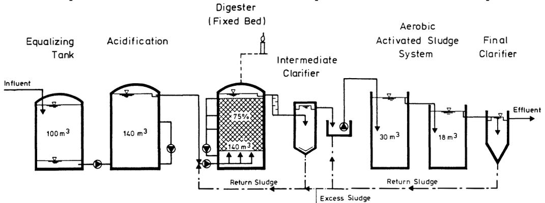
Fig. 1. Flow diagram of molasses distillery anaerobic/aerobic wastewater treatment plant
