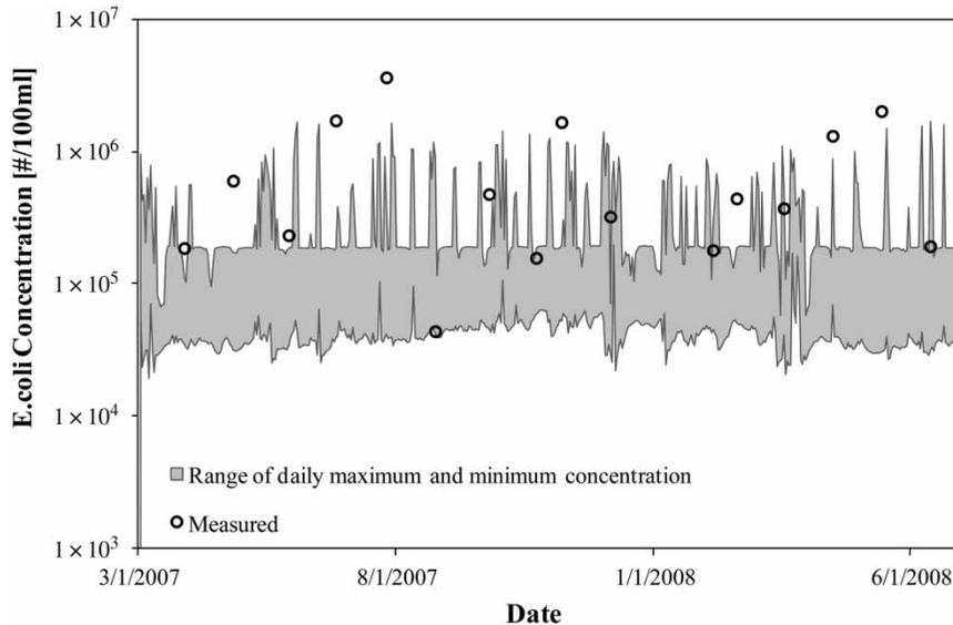
**Figure 9** | Simulated and measured *E. coli* concentration at Leest.
