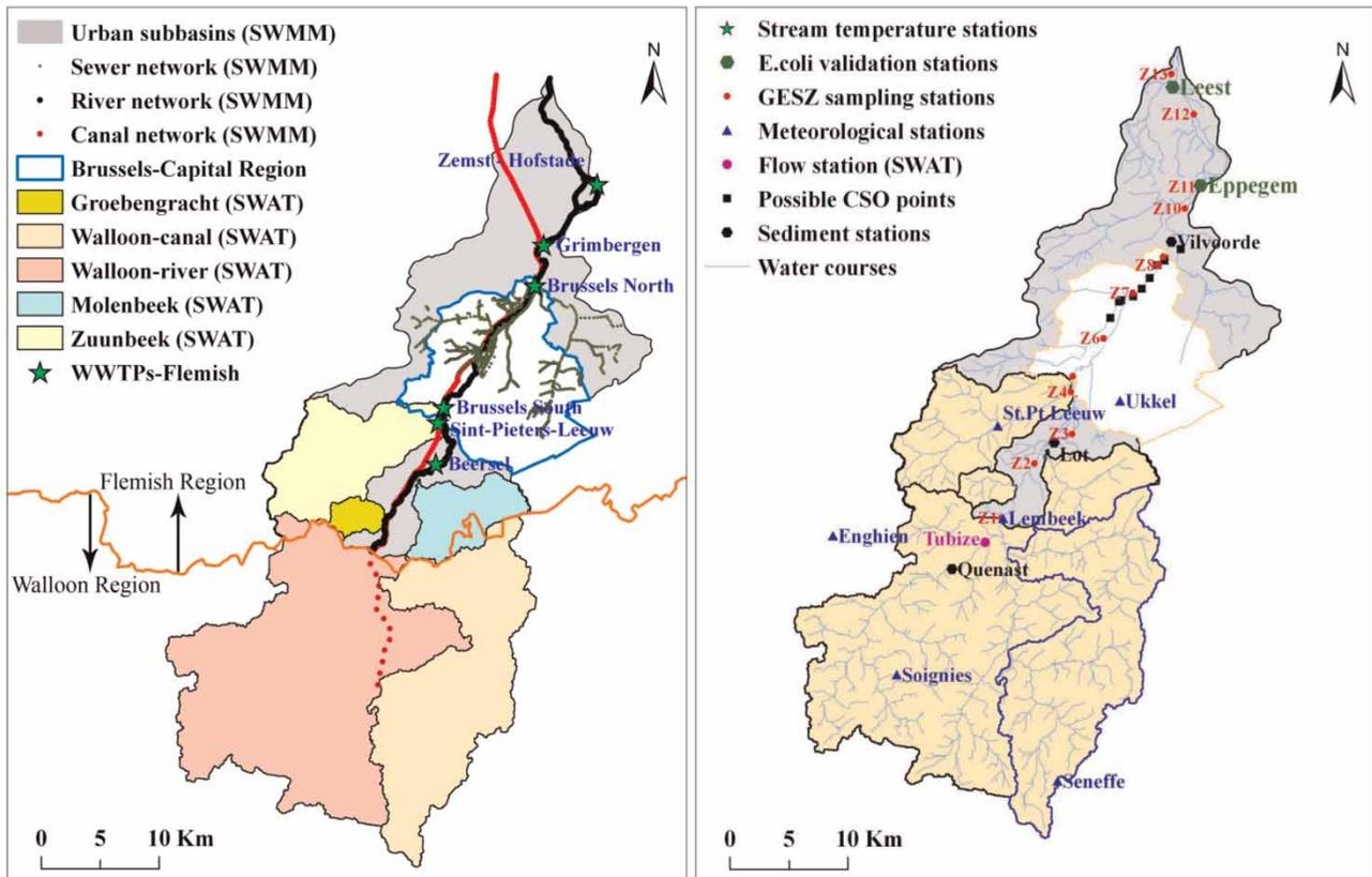
**Figure 1** | The Zenne basin with the subbasins simulated with SWAT, the SWMM network for the river, the canal, the sewer systems and the major WWTPs (left); the hydro-meteorological, stream temperature, *E. coli* validation stations, the GESZ sampling stations and the possible CSO points (right).
