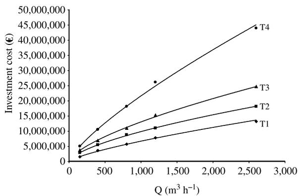
**Figure 3** | Investment cost as a function of wastewater flow rate for the different WWTPs studied.
