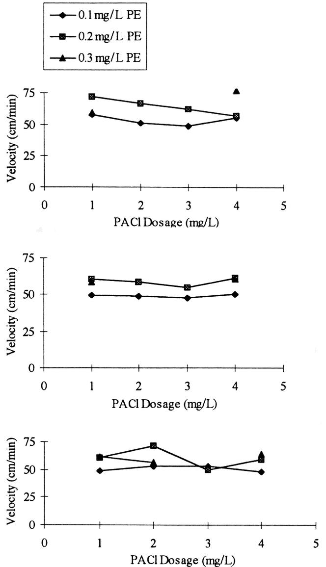
Fig. 5 Pellet-floc settling velocity for the 40 cm/min up-flow velocity condition. Paddle speed: (a) 5 r.p.m., (b) 10 r.p.m., (c) 15 r.p.m.
