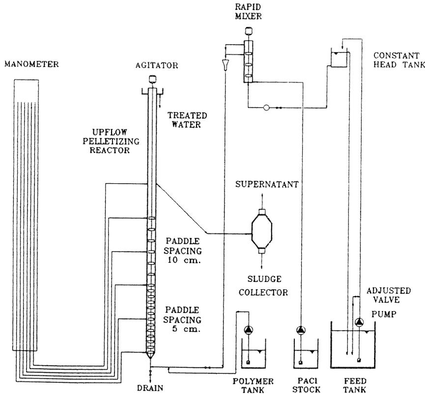
Fig. 1 Diagram of the up-flow pelletisation process setup.
