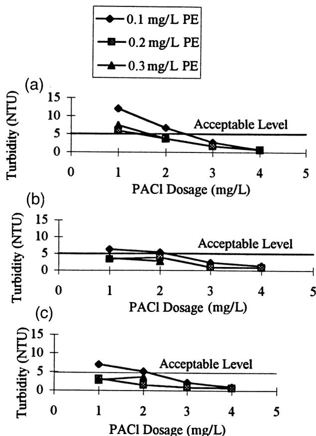
Fig. 2 Effluent turbidity for the 30 cm/min up-flow velocity condition. Paddle speed: (a) 5 r.p.m., (b) 10 r.p.m., (c) 15 r.p.m.
