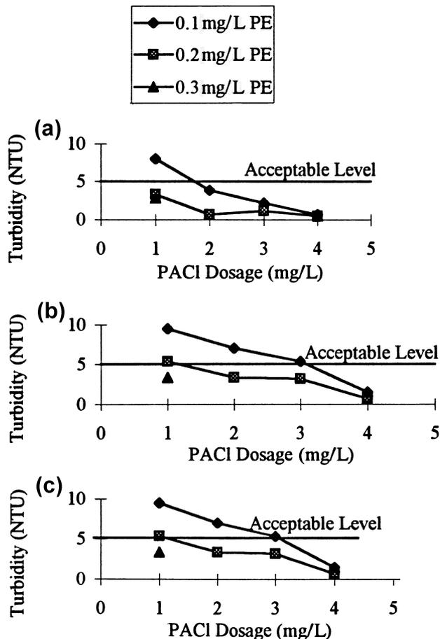
Fig. 3 Effluent turbidity for the 40 cm/min up-flow velocity condition.
