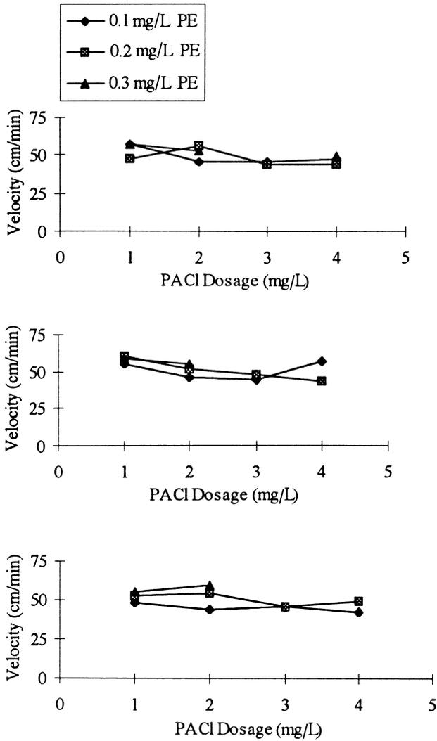
Fig. 4 Pellet-floc settling velocity for 30 cm/min up-flow velocity condition. Paddle speed: (a) 5 r.p.m., (b) 10 r.p.m., (c) 15 r.p.m.
