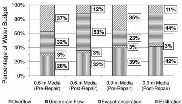
Figure 2 | Partitioning of runoff among overflow, treated underdrain flow, modeled ET, and exfiltration to underlying soil for pre- and post-repair periods.
