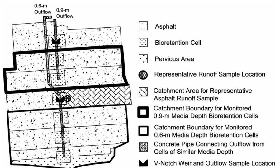
Figure 1 | Layout of catchment and bioretention cells.
