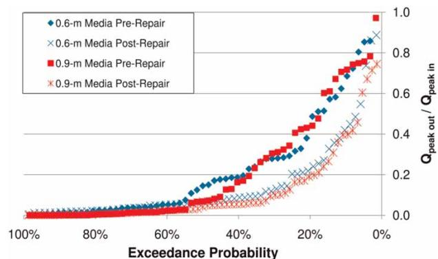
Figure 3 | Peak flow mitigation exceedance probabilities for pre- and post-repair BRCs.
