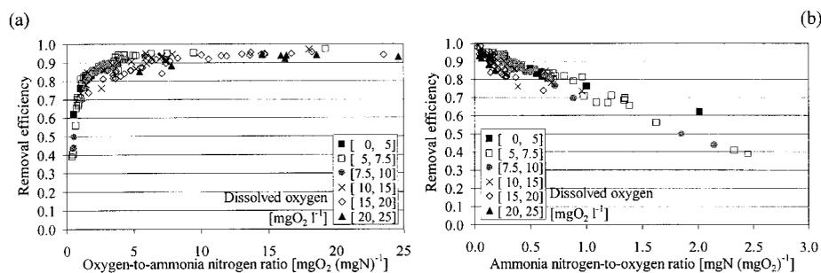
**Figure 3** Removal efficiency versus O/N (a) and N/O (b) ratios
