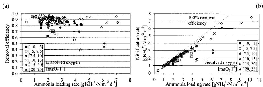
**Figure 2** Removal efficiency (a) and nitrification rate (b) versus ammonia loading rate
