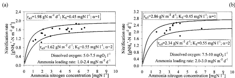
**Figure 5** Nitrification rate versus ammonia nitrogen concentration at different dissolved oxygen concentration: experimental data and calculated kinetics
