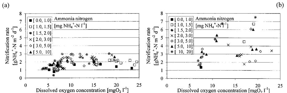
**Figure 4** Nitrification rate versus dissolved oxygen concentration at low-loading (a) and high-loading (b) conditions
