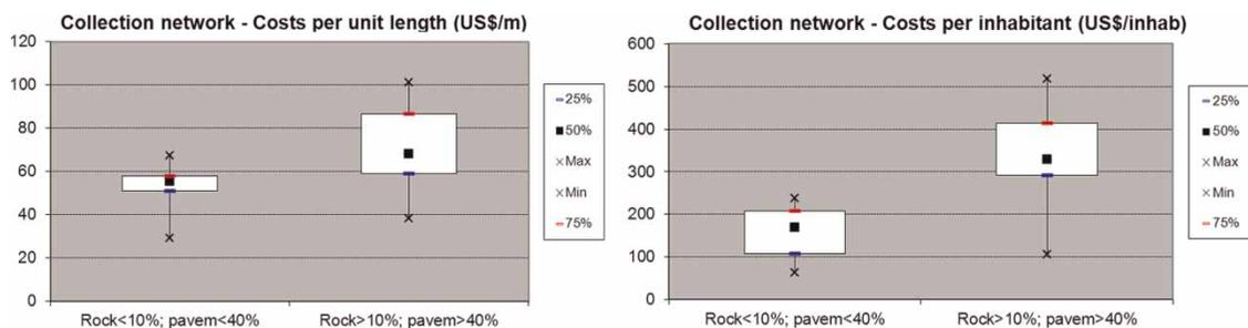
**Figure 3** | Construction costs for the sewerage collection network, expressed as capital costs per unit length (US\$/m) and per inhabitant (US\$/inhabitant) (base year: 2010).
