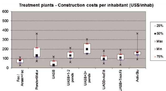
**Figure 6** | Construction costs for the wastewater treatment plants as a function of the treatment process, expressed as capital costs per inhabitant (US\$/inhabitant) (base year: 2010).
