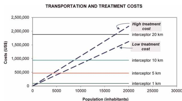
**Figure 9** | Capital costs for transportation (solid horizontal lines) and treatment (dashed lines), for different combinations. Data are the same as the one presented in the example in the text (interceptor costs = US\$94/m; low treatment costs = US\$81/inhabitant; high treatment costs = US\$109/inhabitant).
