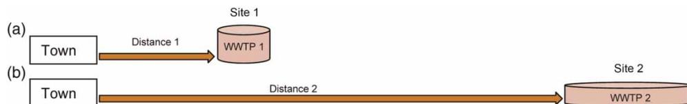
**Figure 8** | Two common alternatives in preliminary studies. (a) Smaller and cheaper interceptor, more compact and more expensive treatment (site 1). (b) Larger and more expensive interceptor, natural and less expensive treatment (site 2).
