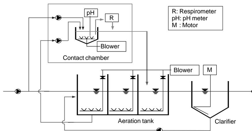
Figure 1 The pilot plant equipped with the inhibition detection system
