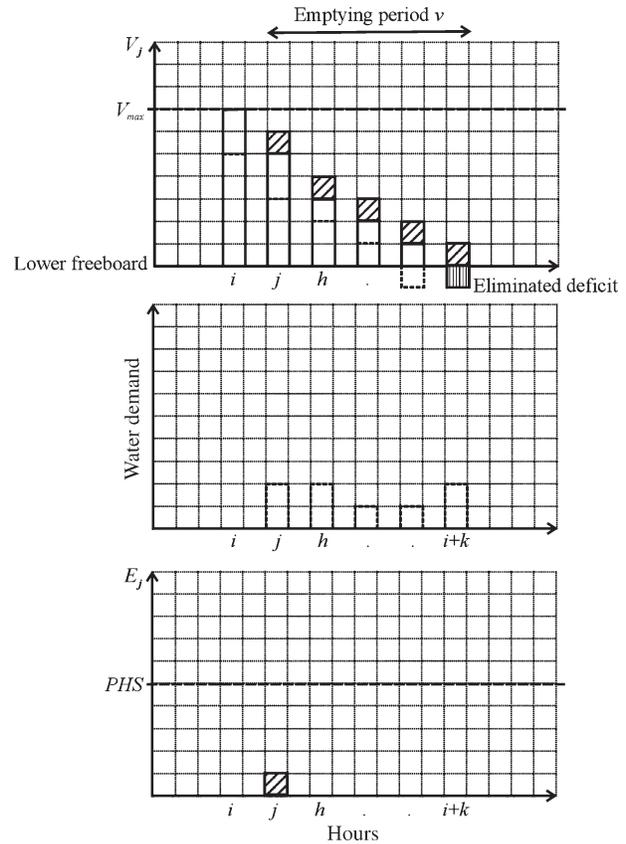
**Figure 3** | Volume to be pumped at hour  $j$  ( $E_{j,v} = \Delta V_{j,v}$ ) conditioned by the deficit at the end of the emptying period  $v$  (hour  $i + k$ :  $-V_{i+k,v}$ ). The deficit is eliminated, thus satisfying demand during the emptying period  $v$ :  $\Delta V_{j,v} = -V_{i+k,v}$ . Hour  $j$  corresponds to the lowest energy tariff during the given emptying period  $v$ .
