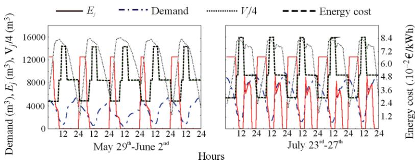
**Figure 9** | Optimal operating scheme for the first pumping station with regulating reservoir having two operating cycles (represented to scale  $V_j/4$ ).
