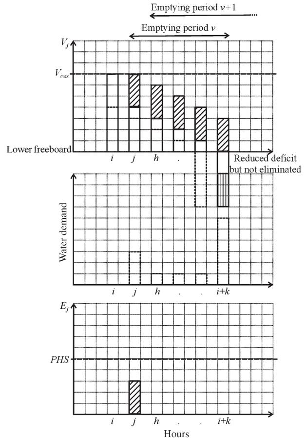
**Figure 5** | Volume to be pumped conditioned by lower deficit volume ( $VR_{j,v}$ ) between the hour selected for pumping (hour  $j$ ) and the final hour of the emptying period  $v$  (hour  $i+k$ ). Deficit was not eliminated at final hour ( $-V_{i+k,v}$ ), but has been reduced:  $\Delta V_{j,v} = VR_{j,v}$ . Hour  $j$  corresponds to the lowest energy tariff during the given emptying period  $v$ .
