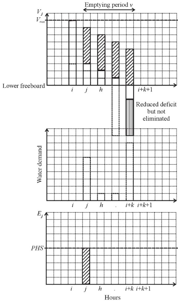
**Figure 4** | Volume to be pumped at hour  $j$  ( $E_{j,v} = \Delta V_{j,v}$ ) conditioned by the potential hourly supply (PHS). Deficit at hour  $i+k$  ( $-V_{i+k,v}$ ) was not eliminated, but has been reduced:  $\Delta V_{j,v} = PHS$ . Hour  $j$  corresponds to the lowest energy tariff during the given emptying period  $v$ .
