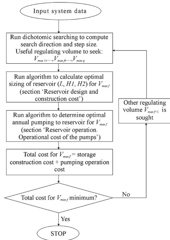
Figure 1 | Flow chart of the optimization model.
