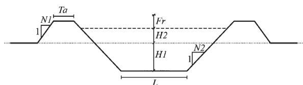
**Figure 2** | Regulating reservoir cross-section and parameters.
