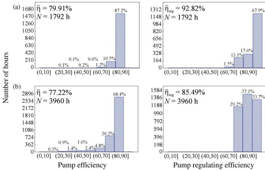
**Figure 10** | Frequency distribution of pump efficiencies ( $\eta$ ) and pump regulating efficiencies ( $\eta_{reg}$ ) for the first pumping station: a) with regulating reservoir and b) without regulating reservoir ( $N$  = number of pumping hours).
