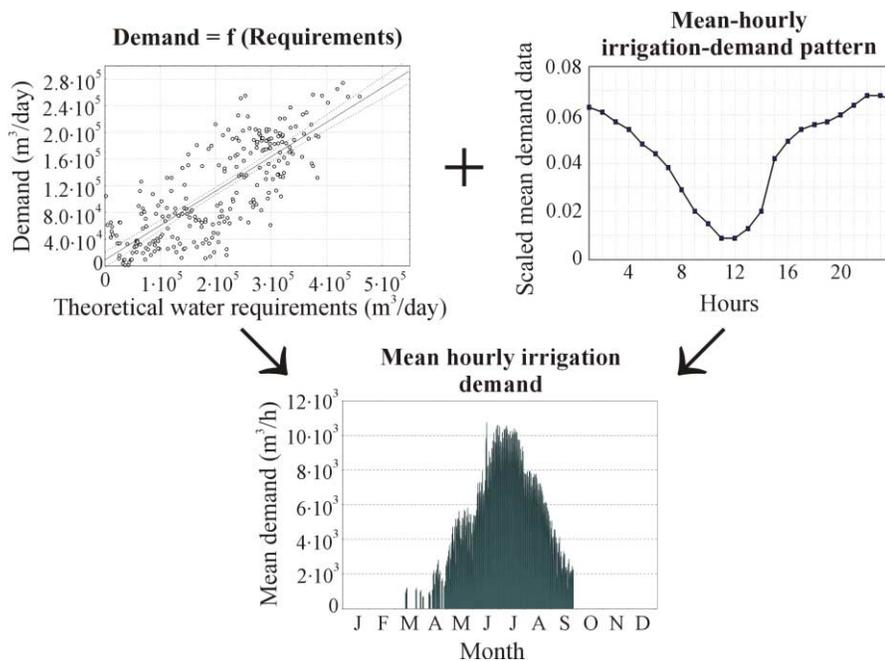
Figure 8 | Disaggregation of daily water demand to hourly demand using the mean-hourly irrigation-demand pattern.
