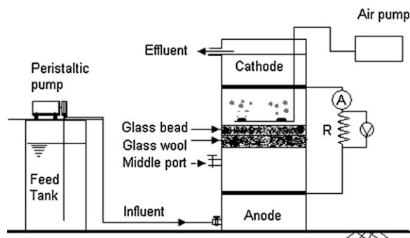
Figure 1 | Membrane-less microbial fuel cell used in the study.
