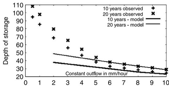
**Figure 5** Calculation of critical volume by simulation of all events (points), and by the conditional model (lines) for 10 and 20 years return period as a function of basins discharge in mm/hour
