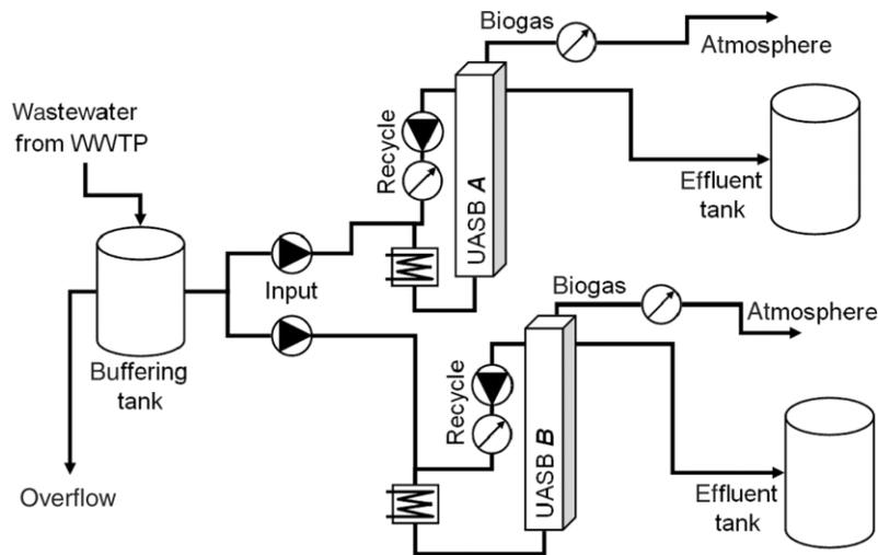
**Figure 1** Flow scheme of the pilot plant at ISAH experimental place
