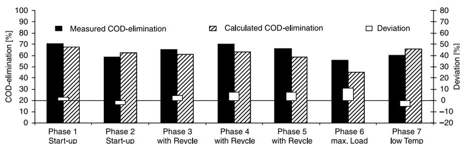
**Figure 4** Comparison between measured and calculated COD removal
